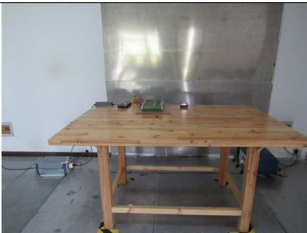
Conducted Emissions Test Setup Front View
