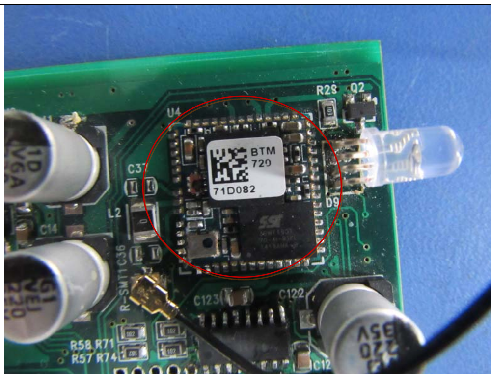
Antenna Module Front View
