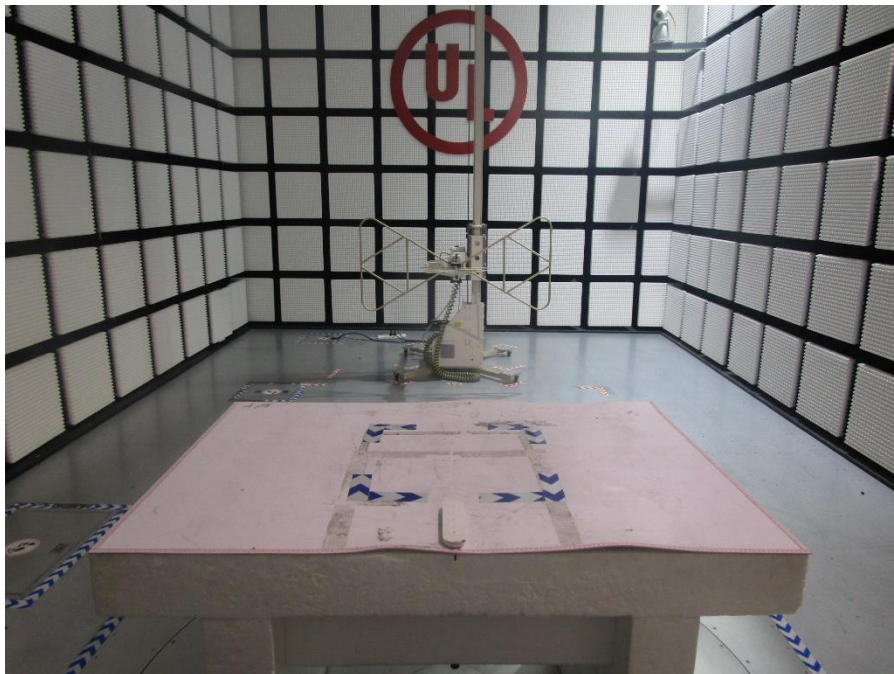
RADIATED RF MEASUREMENT SETUP (Below 1 GHz)
