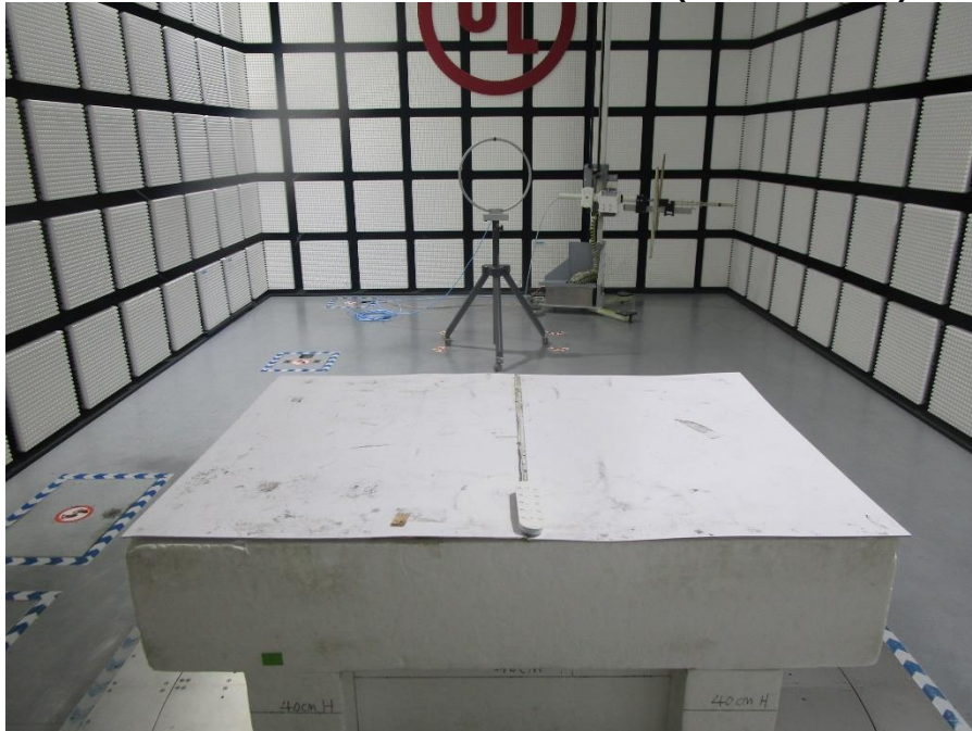
RADIATED RF MEASUREMENT SETUP (Below 1 GHz)
