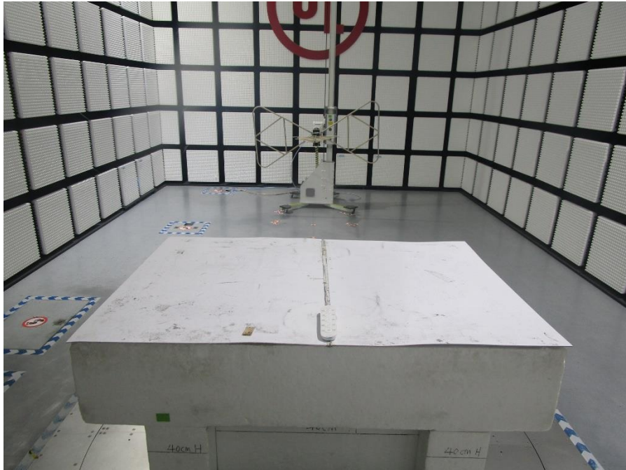
RADIATED RF MEASUREMENT SETUP (Below 1 GHz)
