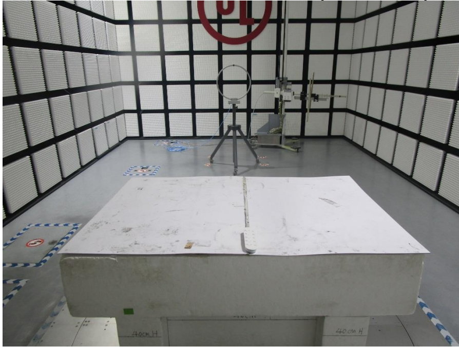
RADIATED RF MEASUREMENT SETUP (Below 1 GHz)
