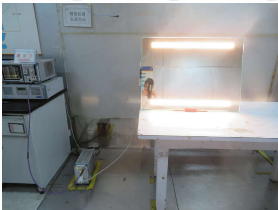
Conducted Emissions Test Setup
