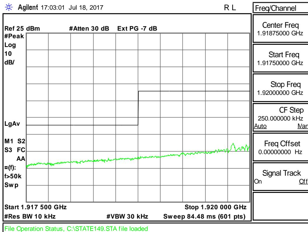
Out-of-band Unwanted Emissions: CH F<sub>L</sub>
