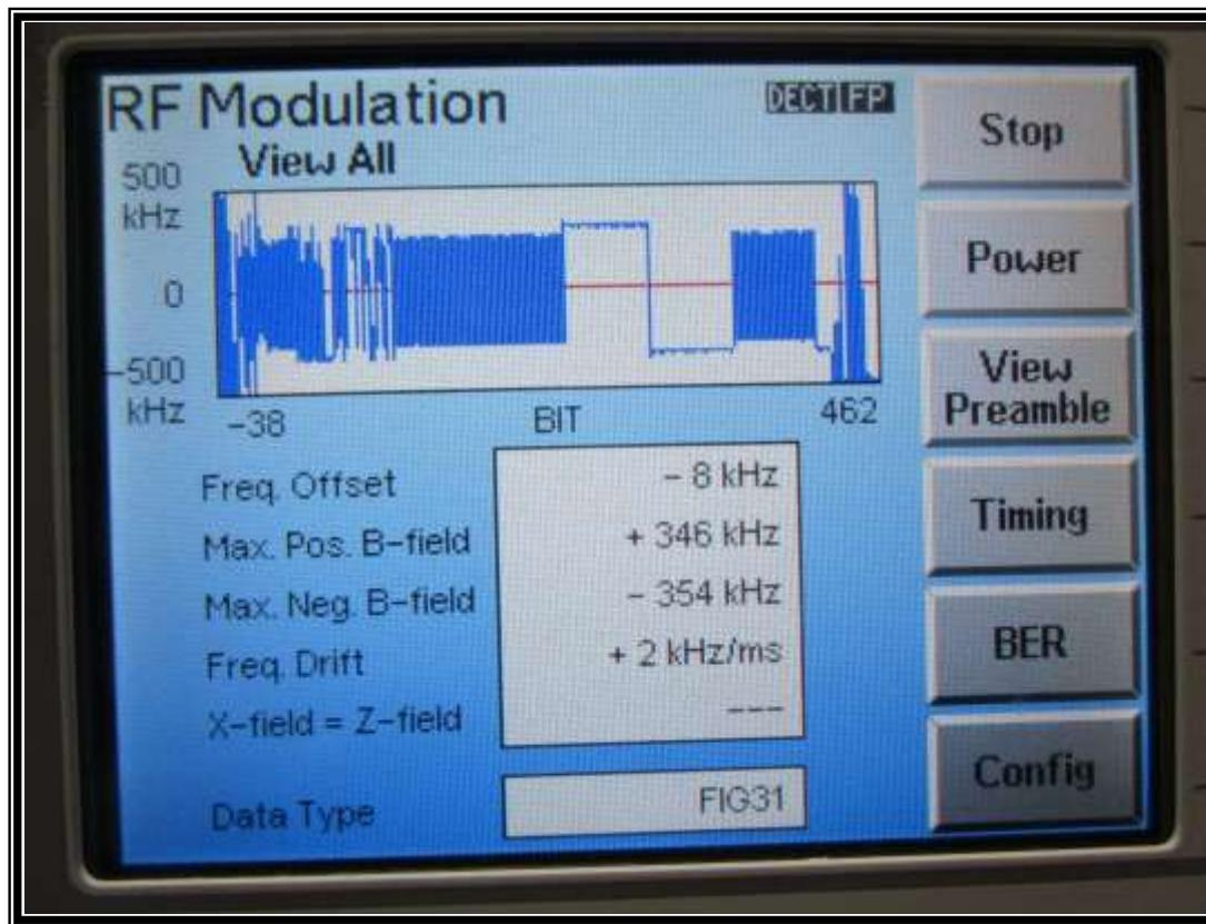
**b) Carrier Frequency Stability over AC adapter power supply voltage**
