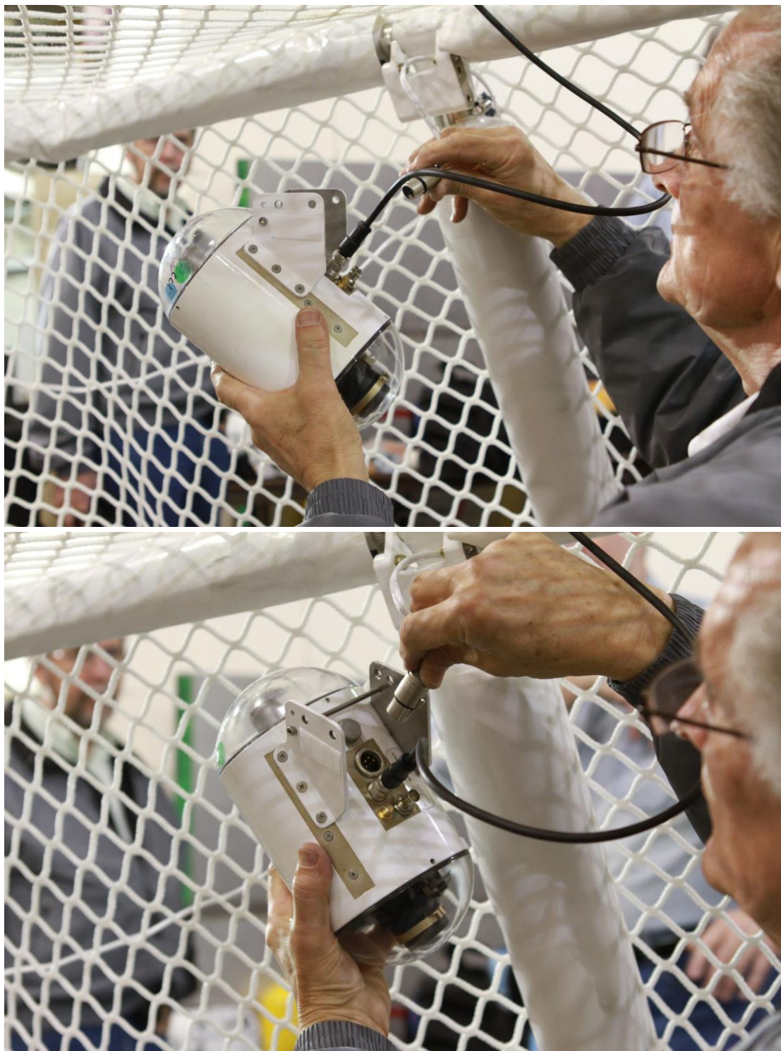
Connect Auxiliary Batter Cable and Data Cable to GoalCam-TX
