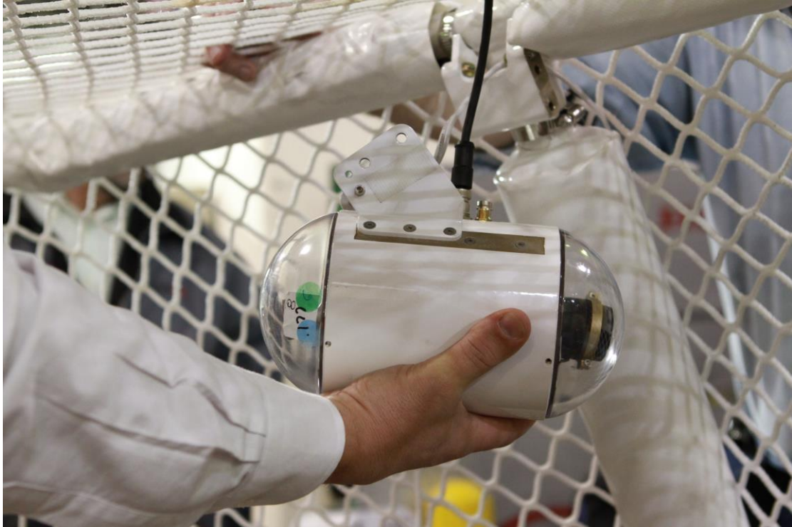
Mount GoalCam-TX to Mounting Bracket Using 1 or 2 Fixed Ball Lock Pins
