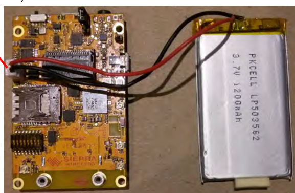
Figure 3-5: mangOH Yellow With Rechargeable Battery Connected
