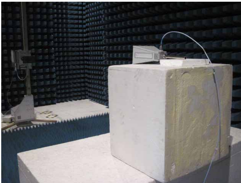
Description: Substitution Antenna for EIRP Test
