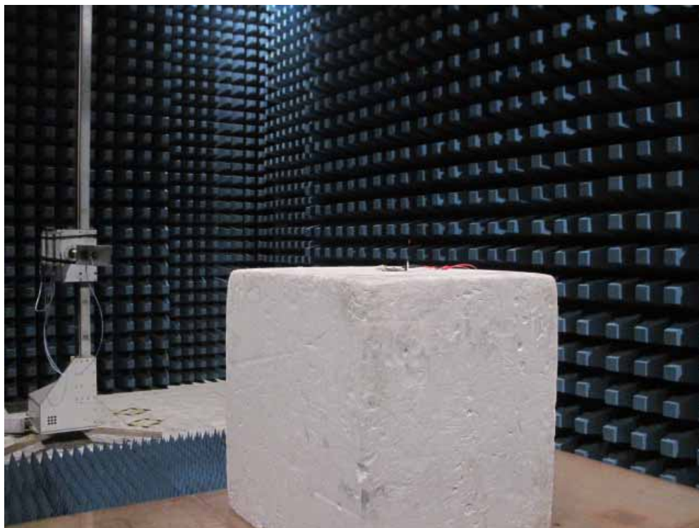
Description: EIRP Test Setup
