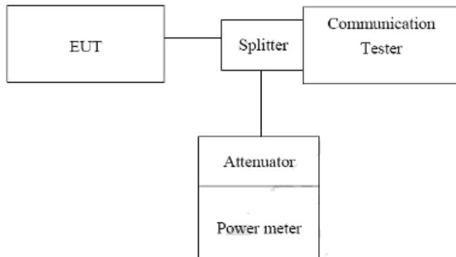
Measurement Setup for testing on Antenna connector.
