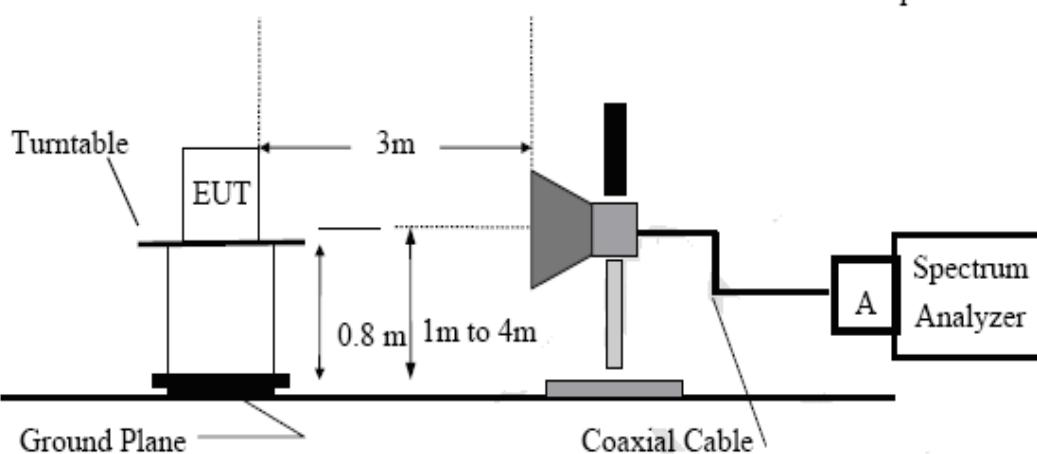
**(C) Substituted Method Test setup:**
