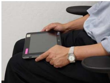
Slate positioned horizontally, with Power Reduction on Cellular. Wi-Fi is transmitting at maximum power
