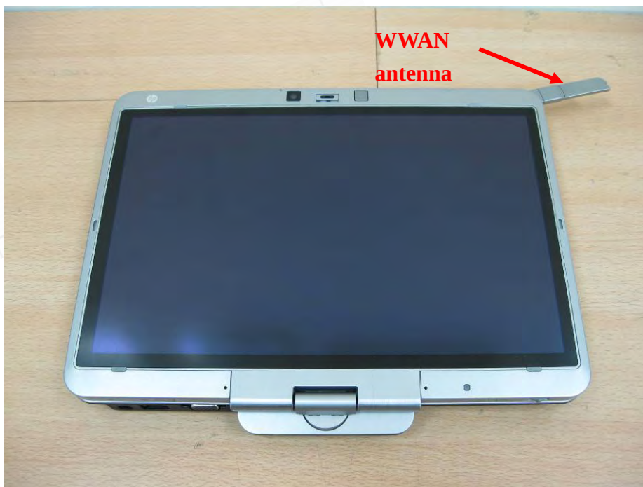
Fig.3 Antenna position of EUT
