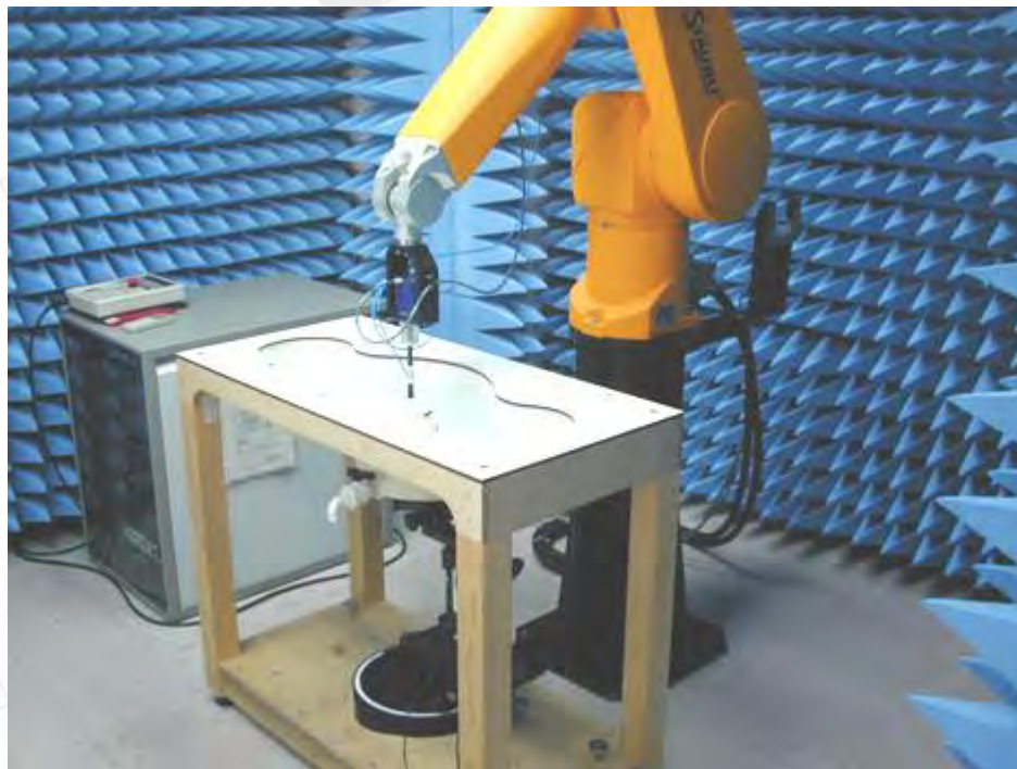
Fig.1 Photograph of the SAR measurement System
