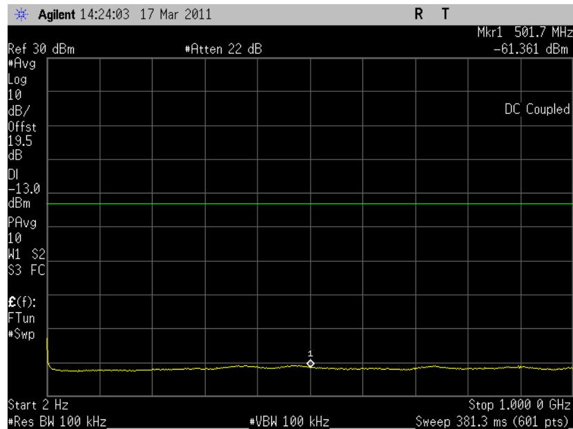
6.3.2.8 *Out of Band Emissions at Antenna Terminals WCDMA, Low channel, 1852.4 MHz, 1 GHz to 20 GHz*
