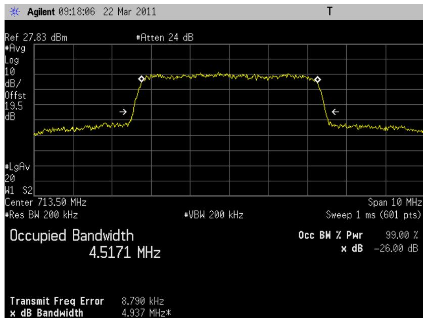
5.3.7.6 *LTE Occupied Bandwidth, Band17 channel (23790) BW=10MHz RB=50 RB Offset=0 QPSK 99% BW*
