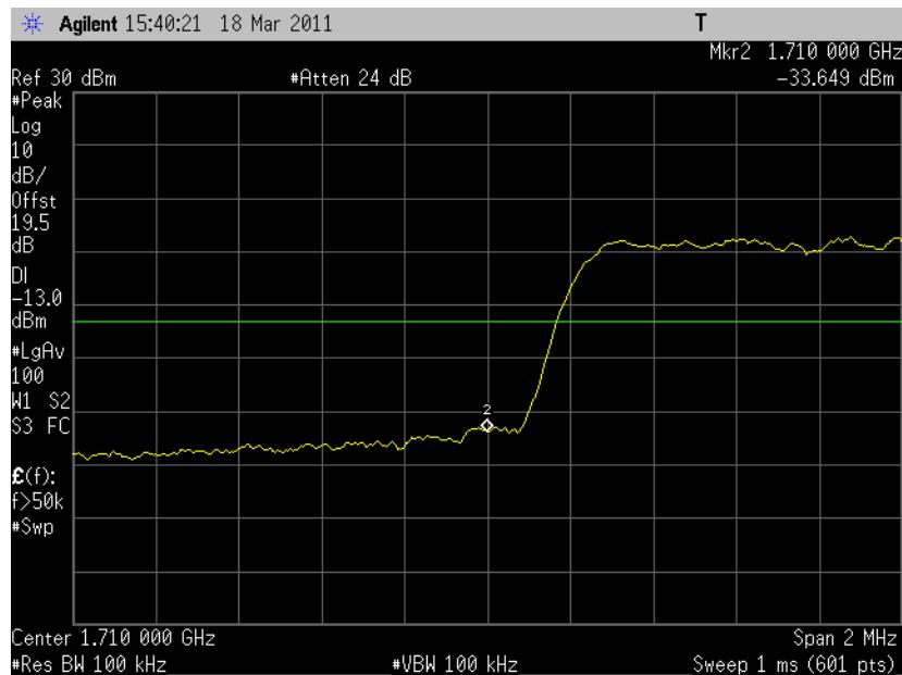
7.3.3.8 *LTE; Band4 above 1755 MHz, with ch20375, 5MHz, 16QAM, 25RB*
