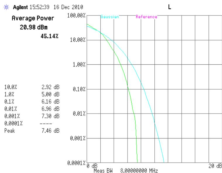
10.4.1.15     *LTE peak to average ratio, 16QAM Band4, mid channel, 1732.5 MHz, 10MHz BW, 50RB*
