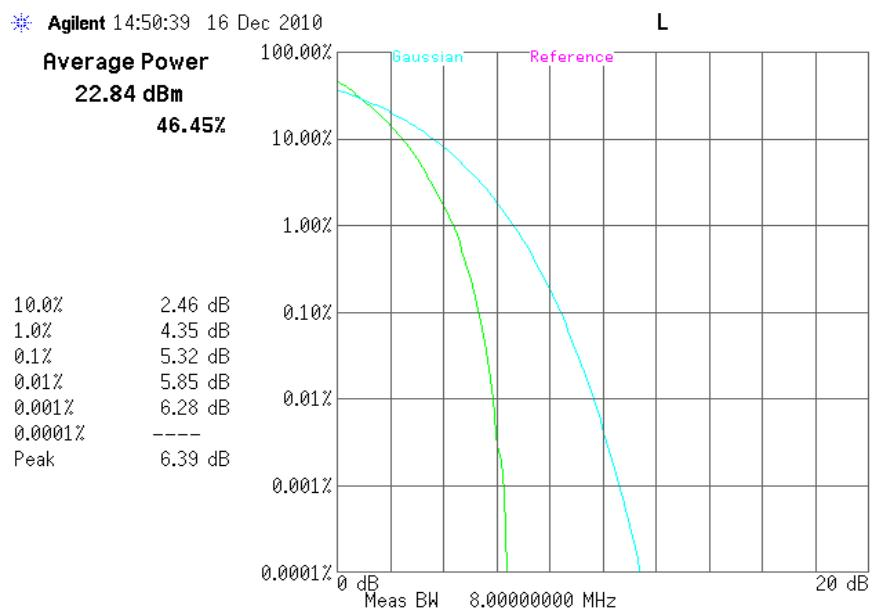
10.4.1.5 LTE peak to average ratio, 16-QAM Band17, Low channel, 706.5 MHz, 5MHz BW, 25RB
