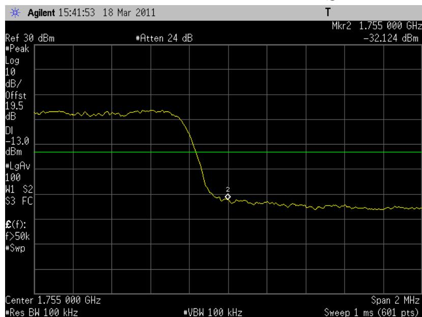
7.3.3.7 *LTE; Band4 below 1710 MHz, with ch19975, 5MHz, 16QAM, 25RB*
