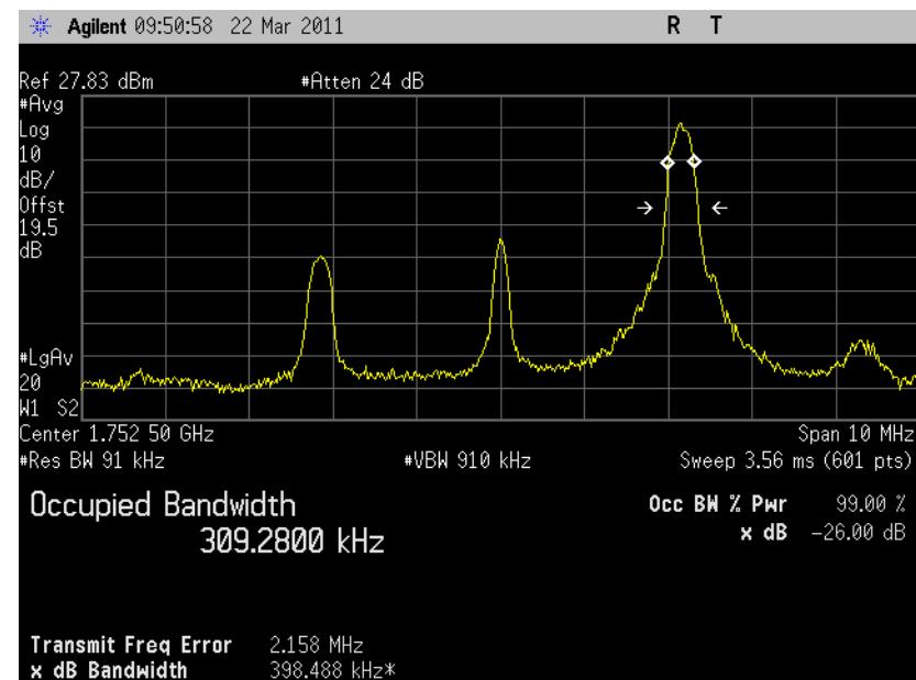
5.3.7.15 LTE Occupied Bandwidth, Band4 low channel (19975) BW=5MHz RB=25 RB
