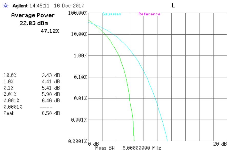
10.4.1.3 *LTE peak to average ratio, QPSK Band17, mid channel, 710 MHz, 10MHz BW, 50RB*
