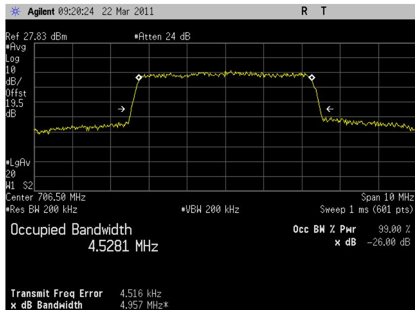
5.3.7.4 *LTE Occupied Bandwidth, Band17 mid channel (23790) BW=5MHz RB=25 RB Offset=0 QPSK 99% BW*
