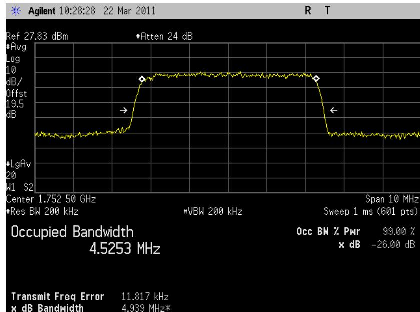
**5.3.7.18 LTE Occupied Bandwidth, Band4 low channel (19975) BW=5MHz RB=1 RB
