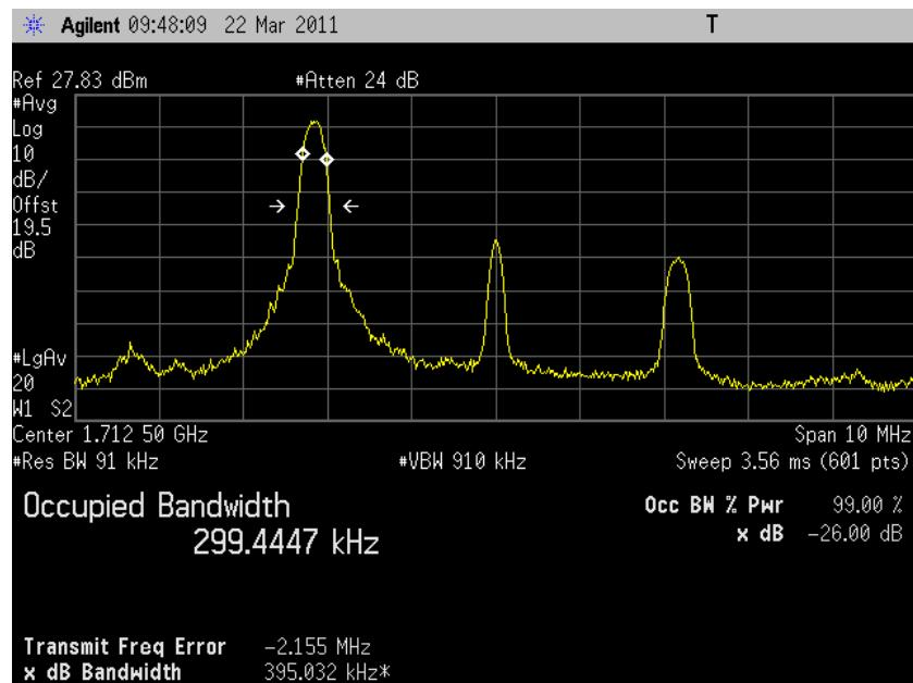
5.3.7.14 LTE Occupied Bandwidth, Band4 high channel (20375) BW=5MHz RB=1 RB
