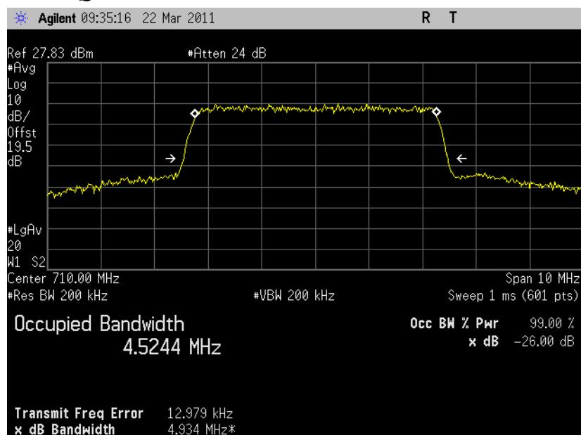
5.3.7.11 LTE Occupied Bandwidth, Band17 high channel (23825) BW=5MHz RB=25
