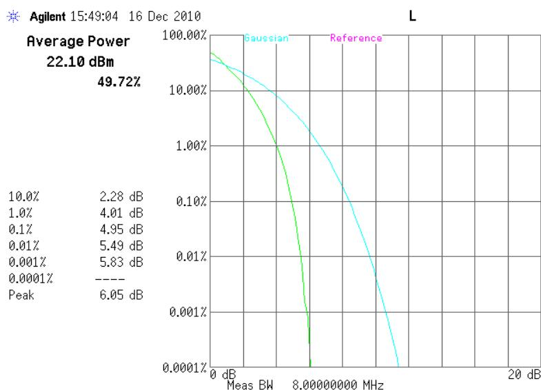
10.4.1.13 *LTE peak to average ratio, 16QAM Band4, low channel, 1712.5 MHz, 5MHz BW, 25RB*
