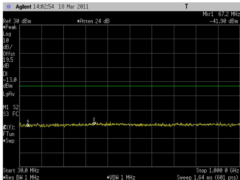
**6.3.3.20 Out of Band Emissions at Antenna Terminals LTE B4, Mid channel, 1732.5 MHz, 5MHz BW, 25RB, QPSK, 1 GHz to 20 GHz**
