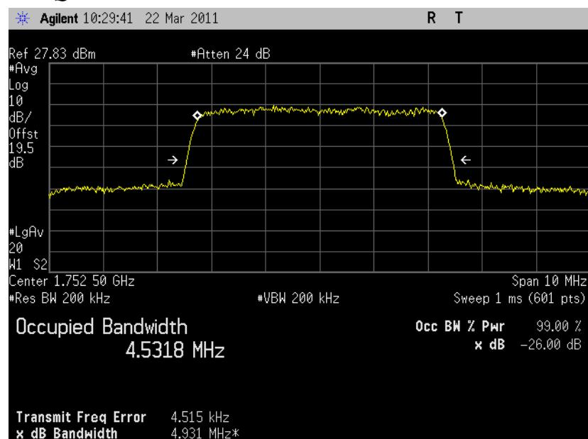
5.3.7.23 *LTE Occupied Bandwidth, Band4 low channel (20000) BW=10MHz RB=50 RB Offset=0 QPSK 99% BW*
