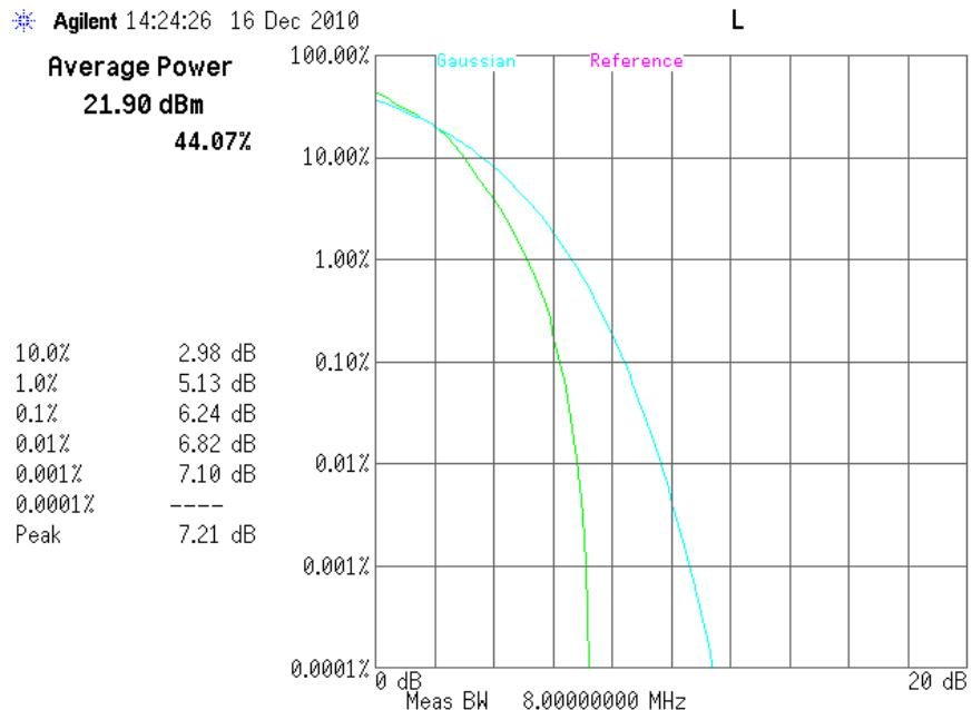
*10.4.1.6 LTE peak to average ratio, 16-QAM Band17, Mid channel, 710 MHz, 5MHz BW, 25RB*
