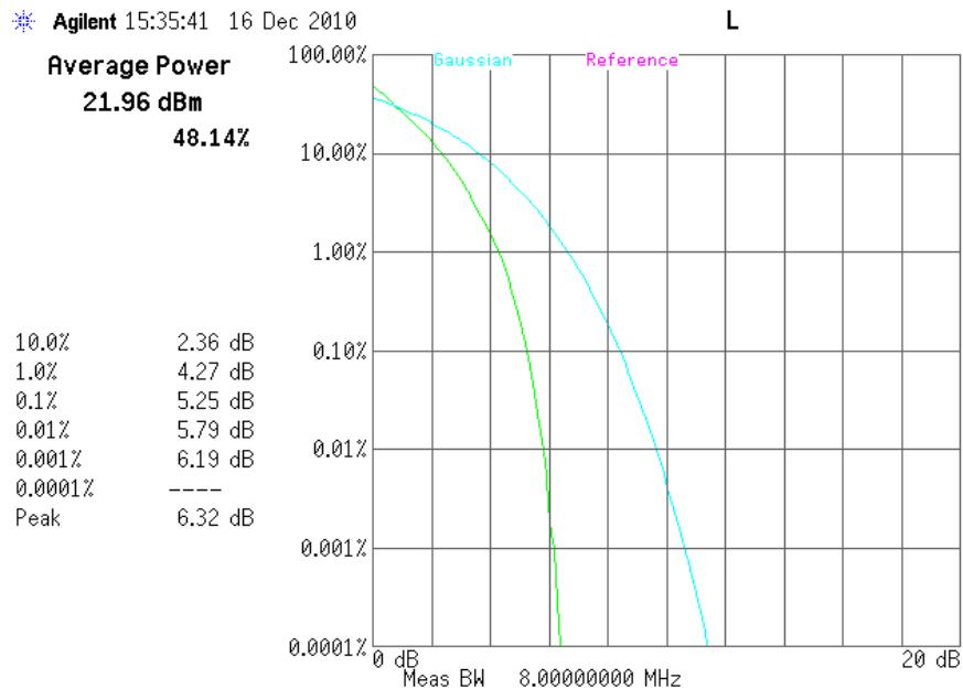
10.4.1.10 *LTE peak to average ratio, QPSK Band4, mid channel, 1732.5 MHz, 5MHz BW, 25RB*
