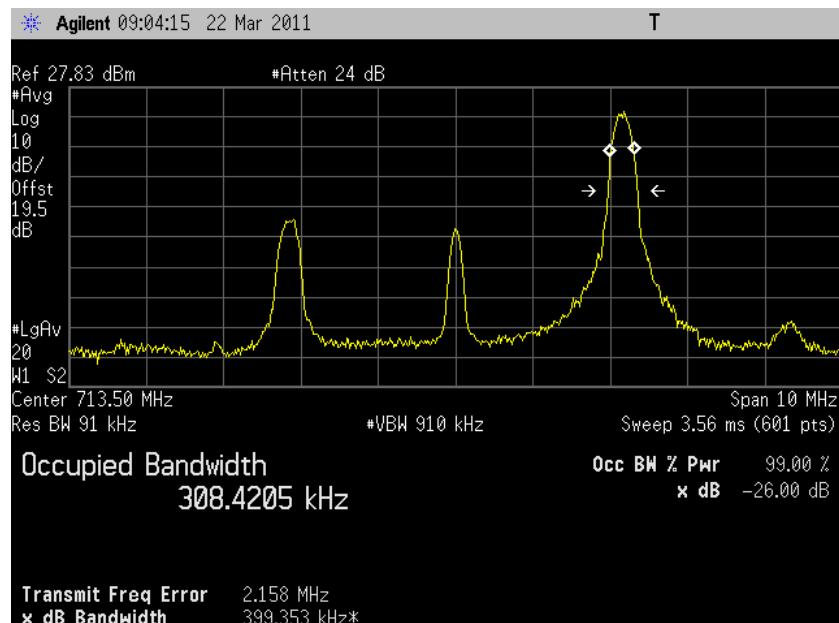
5.3.7.3 *LTE Occupied Bandwidth, Band17 low channel (23755) BW=5MHz RB=25 RB Offset=0 QPSK 99% BW*
