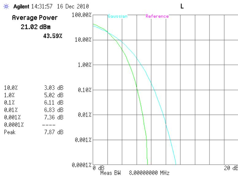
10.4.1.8 LTE peak to average ratio, 16-QAM Band17, high channel, 713.5 MHz, 5MHz BW, 25RB
