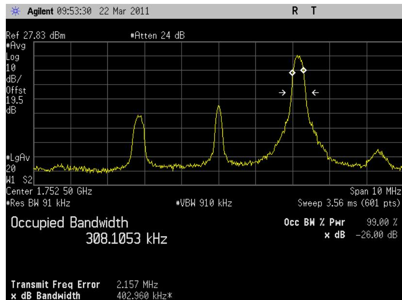
5.3.7.20 LTE Occupied Bandwidth, Band4 low channel (19975) BW=5MHz RB=25 RB
