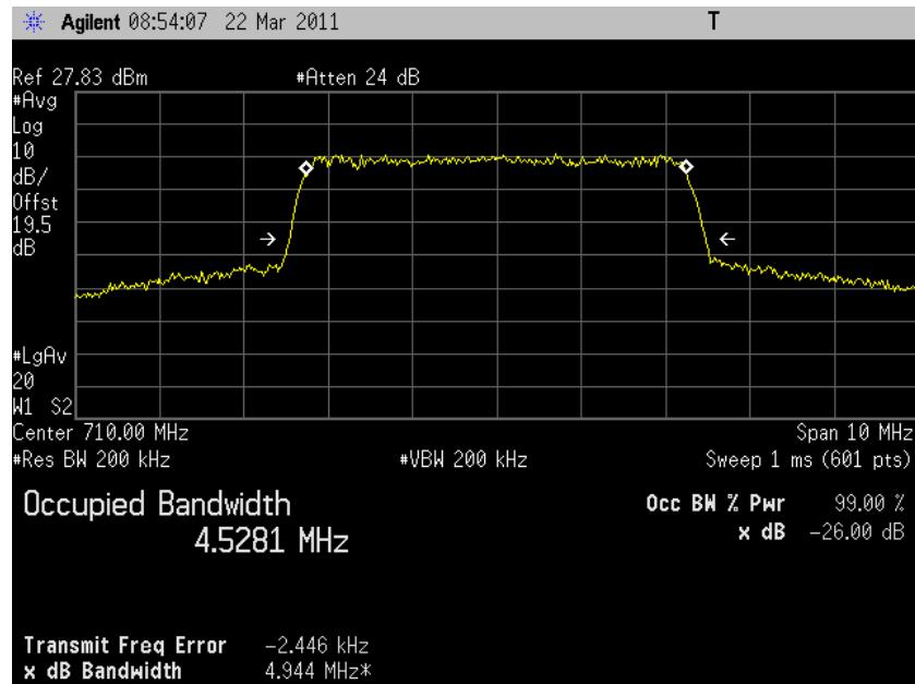
5.3.7.5 *LTE Occupied Bandwidth, Band17 high channel (23825) BW=5MHz RB=25 RB Offset=0 QPSK 99% BW*
