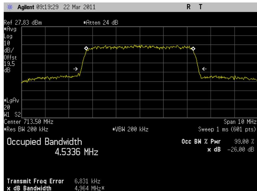
5.3.7.12 LTE Occupied Bandwidth, Band17 mid channel (23790) BW=10MHz RB=50
