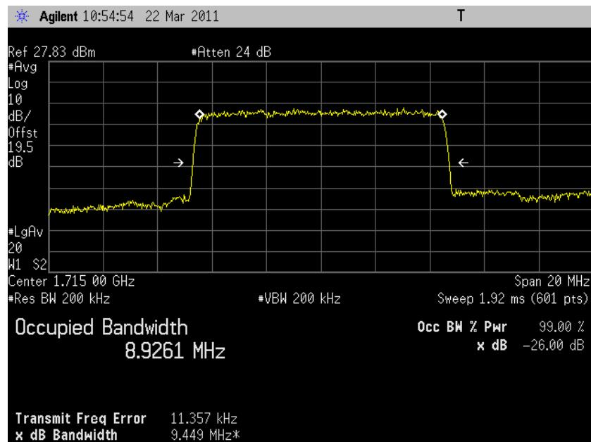
5.3.7.24 *LTE Occupied Bandwidth, Band4 mid channel (20175) BW=10MHz RB=50 RB Offset=0 QPSK 99% BW*
