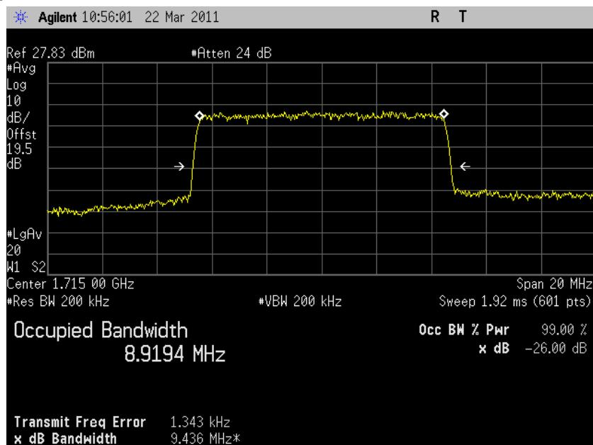
5.3.7.27 *LTE Occupied Bandwidth, Band4 high channel (20734) BW=5MHz RB=25 QPSK 99% BW*
