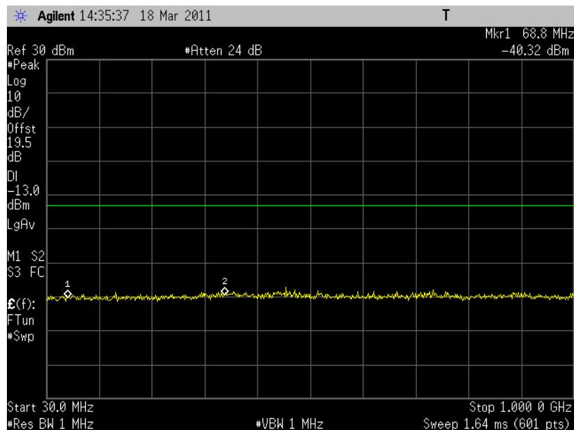
*6.3.3.30 Out of Band Emissions at Antenna Terminals LTE B4, Low channel, 1715.0 MHz, 10MHz BW, 50RB, QPSK, 1 GHz to 20 GHz*
