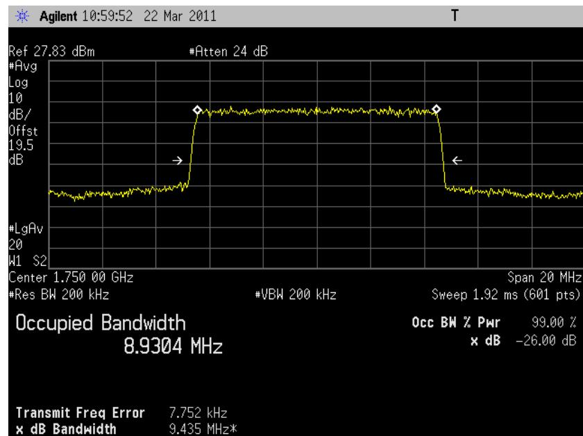
5.3.7.26 *LTE Occupied Bandwidth, Band4 low channel (20000) BW=10MHz RB=50 RB Offset=0 16QAM 99% BW*
