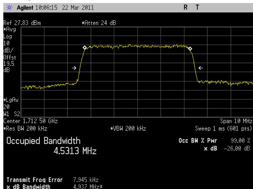
5.3.7.16 LTE Occupied Bandwidth, Band4 mid channel (20175) BW=5MHz RB=25 RB
