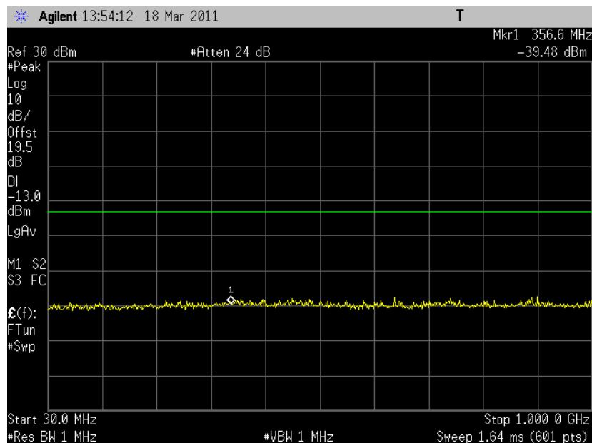
**6.3.3.18 Out of Band Emissions at Antenna Terminals LTE B4, Low channel, 1712.5 MHz, 5MHz BW, 25RB, QPSK, 1 GHz to 20 GHz**
