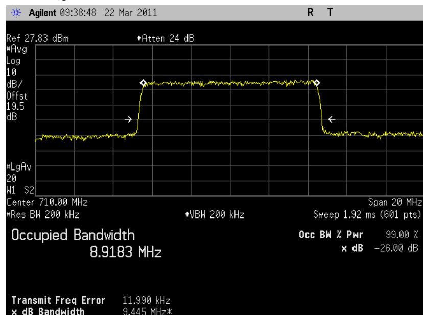
5.3.7.13 LTE Occupied Bandwidth, Band4 low channel (19975) BW=5MHz RB=1 RB
