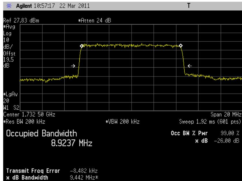
5.3.7.25 *LTE Occupied Bandwidth, Band4 high channel (20350) BW=10MHz RB=50 RB Offset=0 QPSK 99% BW*
