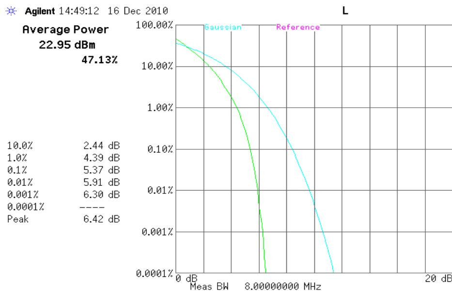
10.4.1.2 *LTE peak to average ratio, QPSK Band17, mid channel, 710 MHz, 5MHz BW, 25RB*
