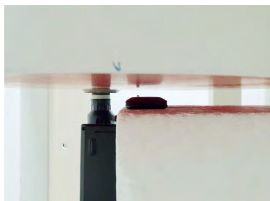
Fig.4 EUT Front side to flat phantom
