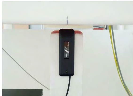
Fig.7 EUT Right side to flat phantom
