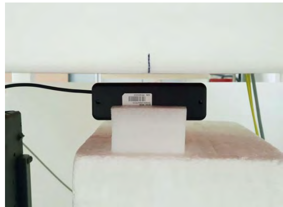
Fig.6 EUT Bottom side to flat phantom
