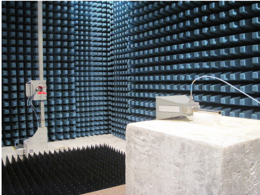
Description: Substitution Antenna for EIRP Test
