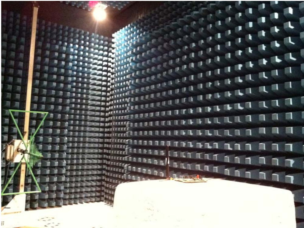
Description: ERP Test Setup
