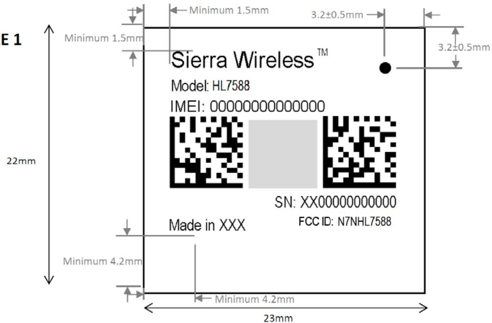
Dimensions are taken with respect to the edge of the surface that the laser etch is made on.
