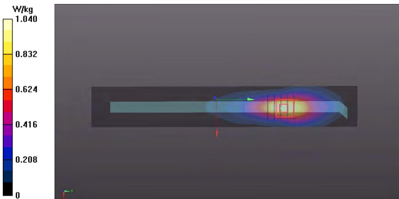
**P23 LTE 25\_QPSK20M\_Top Side\_0cm\_Ch26140\_P sensor w/\_1RB\_OS0****DUT: 150925C05**
