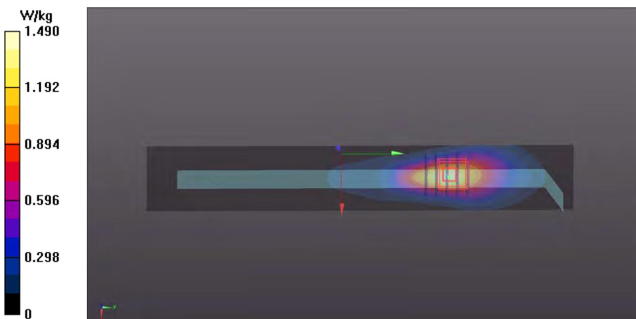
**P17 LTE 2\_QPSK20M\_Top Side\_0cm\_Ch18900\_P sensor w/\_1RB\_OS0****DUT: 150925C05**
