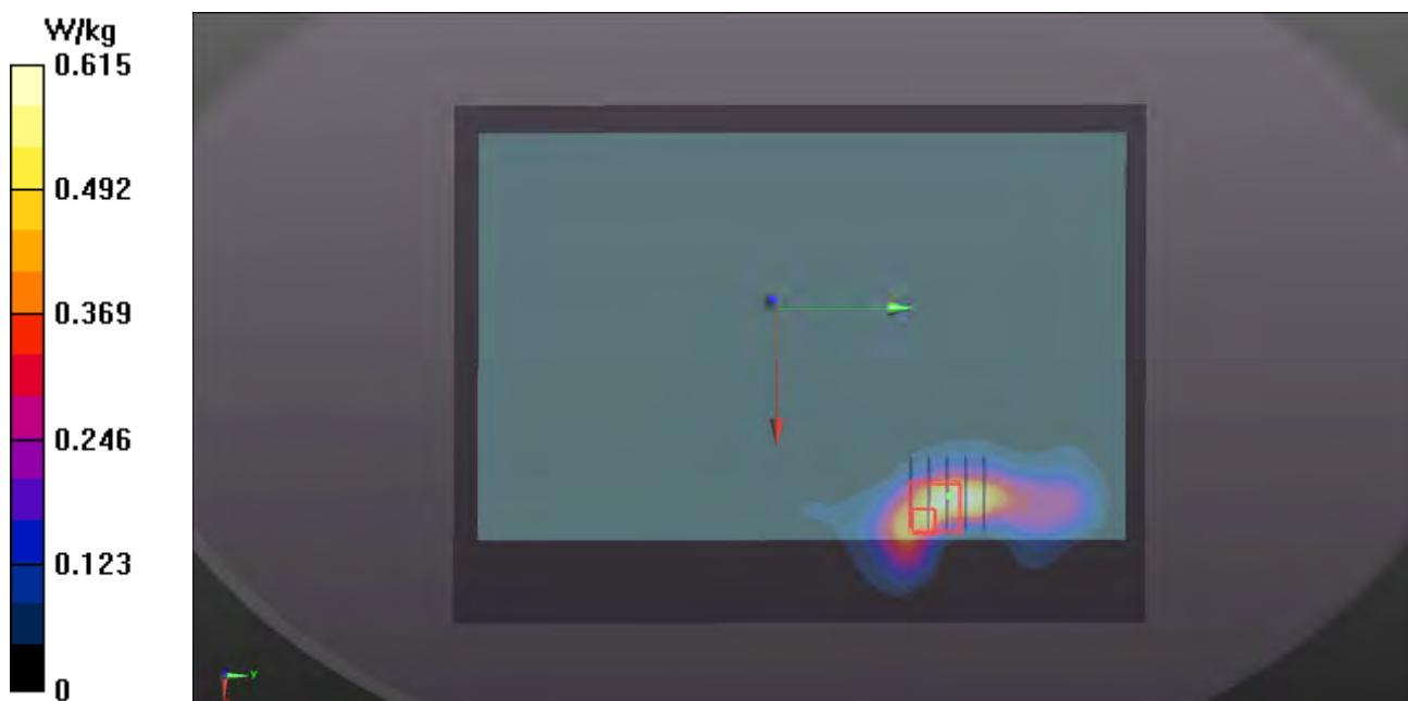
**P13 LTE 41\_QPSK20M\_Top Side\_0cm\_Ch40185\_P sensor w/\_50RB\_OS0****DUT: 150925C05**
