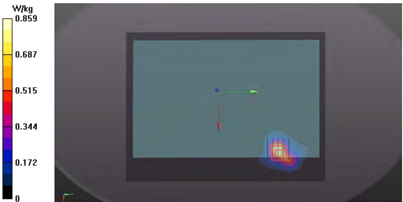
**P11 LTE 26\_QPSK15M\_Top Side\_0cm\_Ch26965\_P sensor w/\_36RB\_OS0****DUT: 150925C05**
