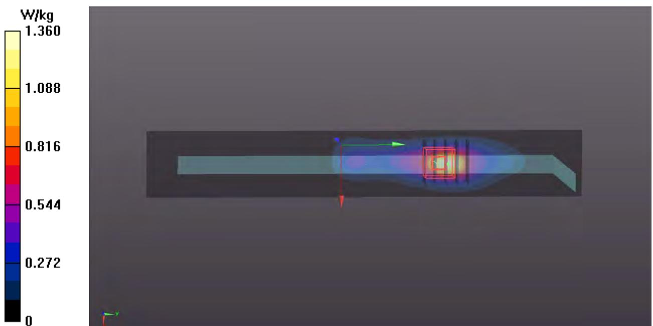
**P26 LTE 41\_QPSK20M\_Top Side\_0cm\_Ch41490\_P sensor w/\_1RB\_OS0****DUT: 150925C05**
