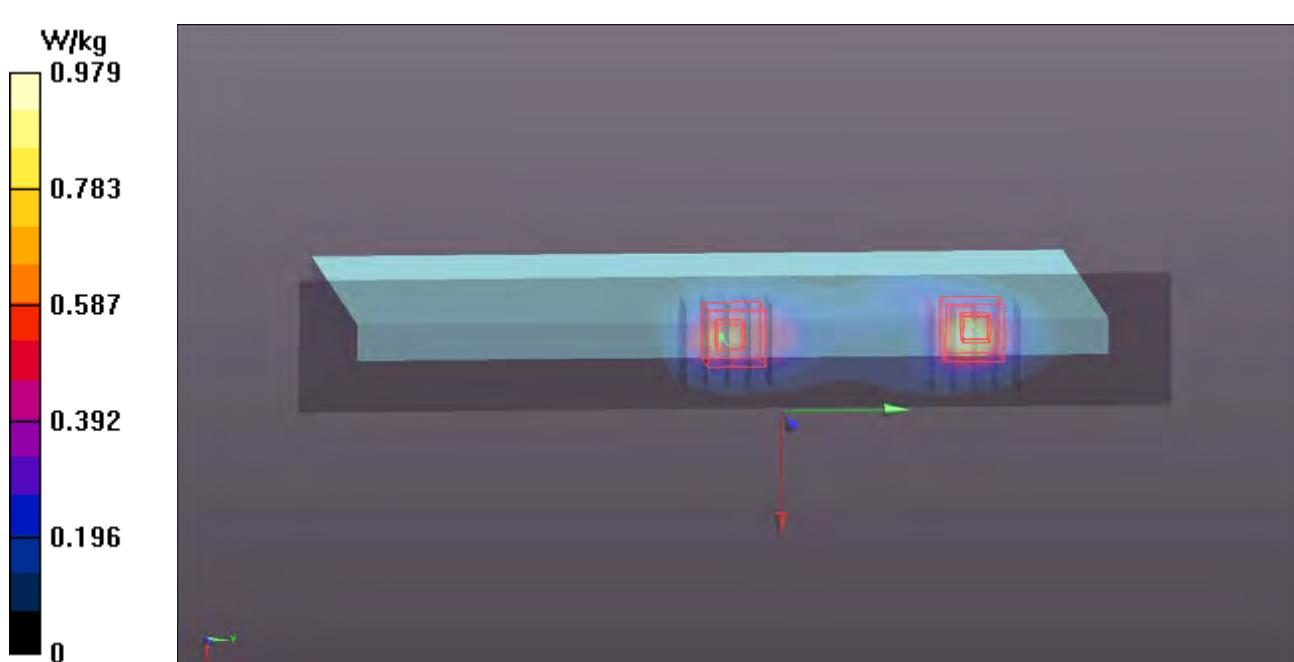
**P24 LTE 26\_QPSK15M\_Top Side\_0cm\_Ch26865\_P sensor w/\_1RB\_OS0****DUT: 150925C05**
