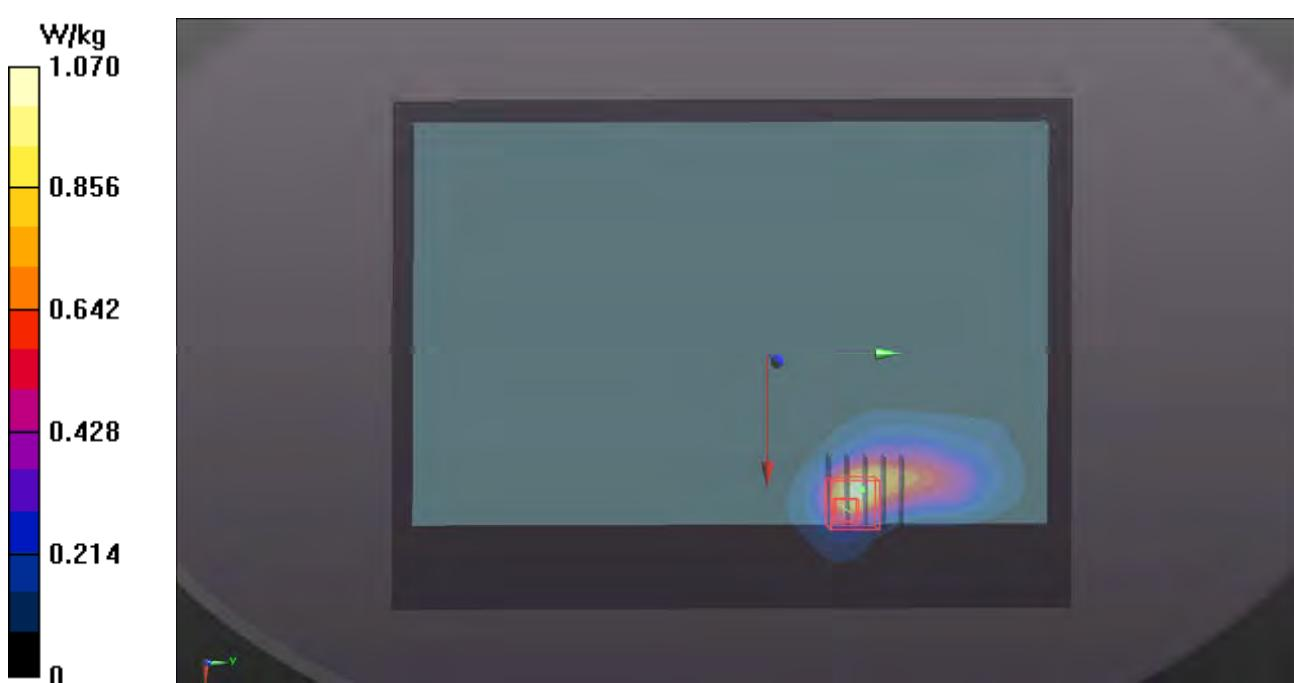
**P08 LTE 12\_QPSK10M\_Top Side\_0cm\_Ch23060\_P sensor w/\_25RB\_OS0****DUT: 150925C05**
