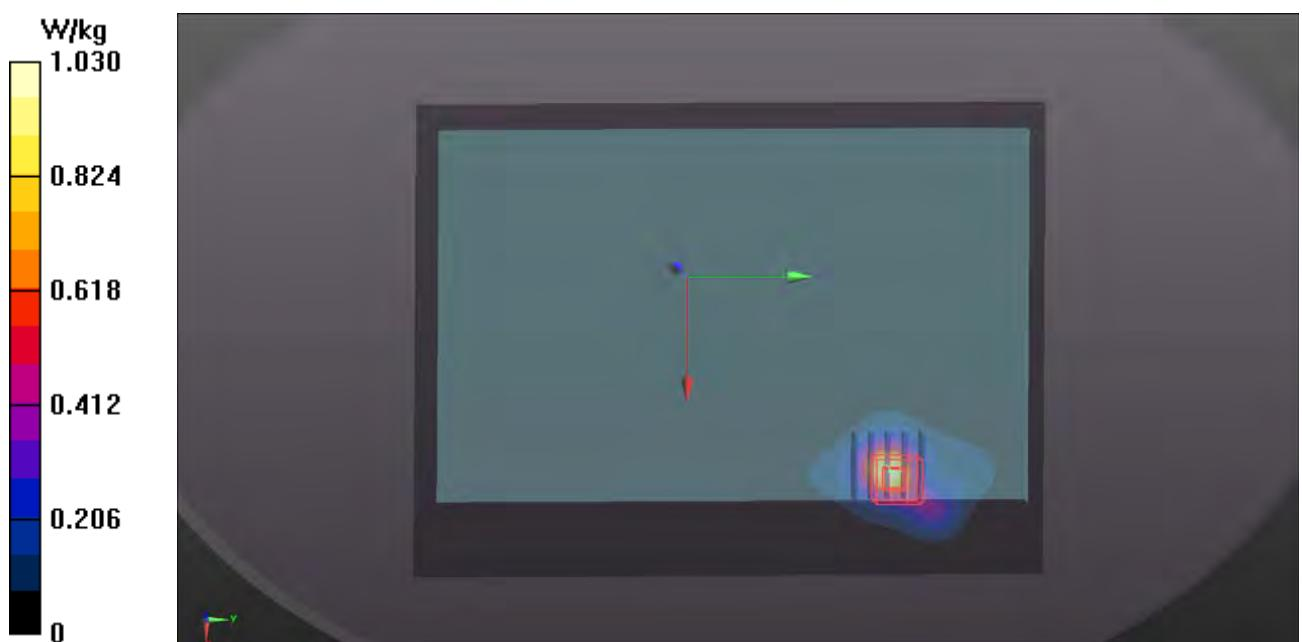
**P05 LTE 4\_QPSK20M\_Top Side\_0cm\_Ch20300\_P sensor w/\_1RB\_OS0****DUT: 150925C05**
