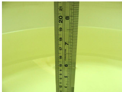
Fig 6.2 Photo of Liquid Height for Body SAR
