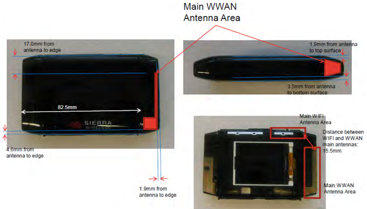
Fig.10 Antenna position of EUT (96.00 x 56.81 x 16.81 mm)
