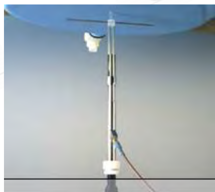
Photograph of the dipole Antenna
