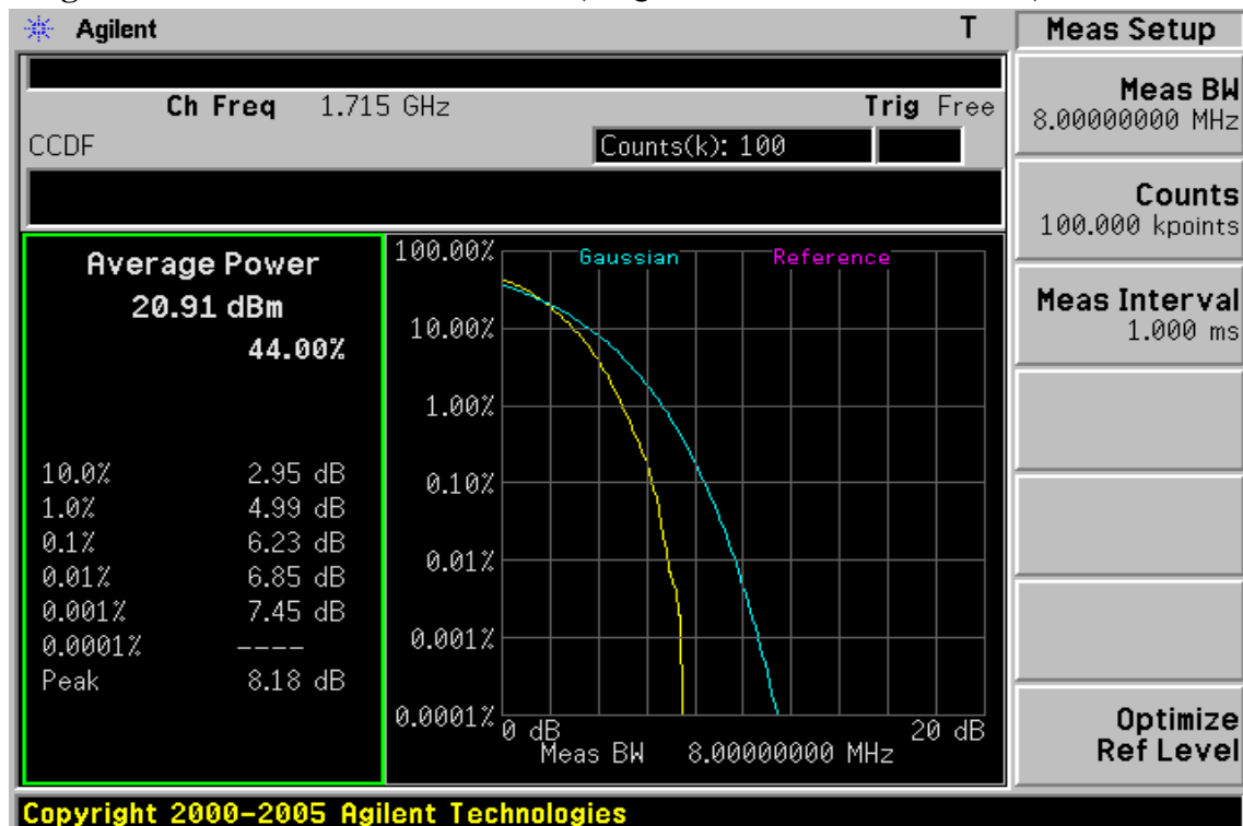
Figure 6-4: 10MHz BW LTE-Band 4(16QAM Number: 50 Offset: 0) Channel Low
