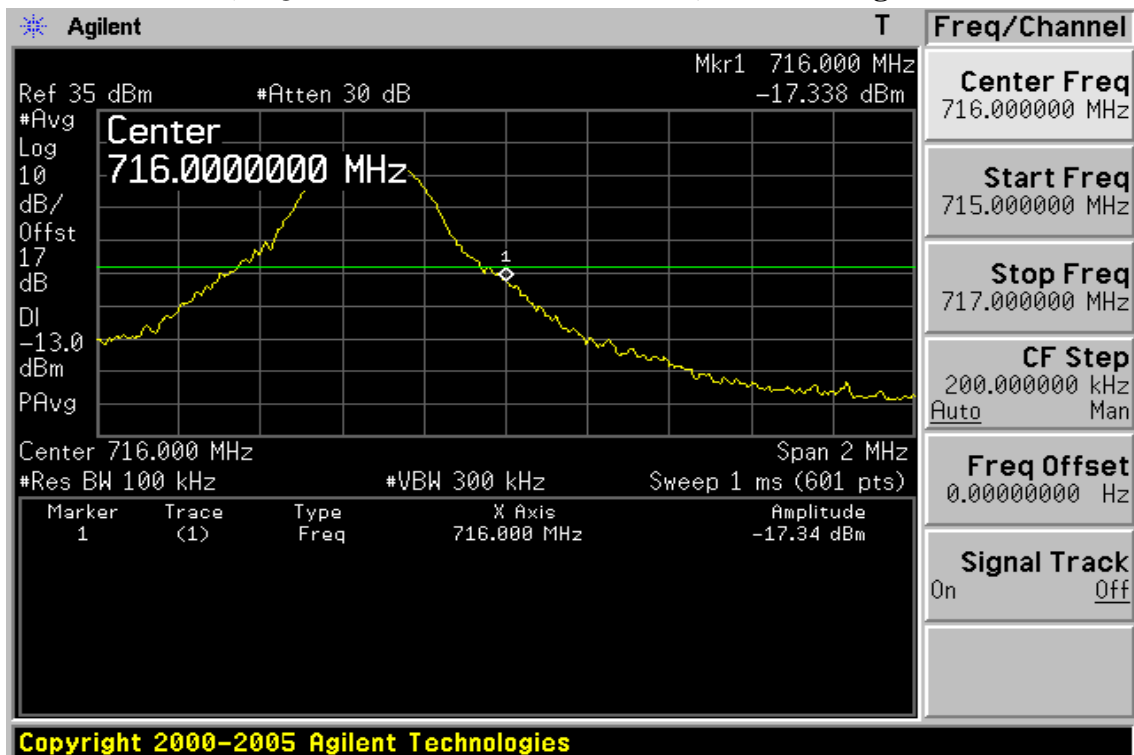
Figure 8-50: Band edge emission at antenna terminals –5MHz BW LTE-Band 17 (16QAM RB Number: 1 Offset: 24) Channel Highest
