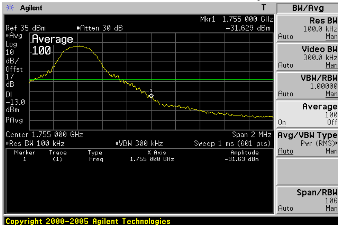
Figure 8-35: Band edge emission at antenna terminals –10MHz BW LTE-Band 4 (QPSK RB Number: 1 Offset:49) Channel Highest
