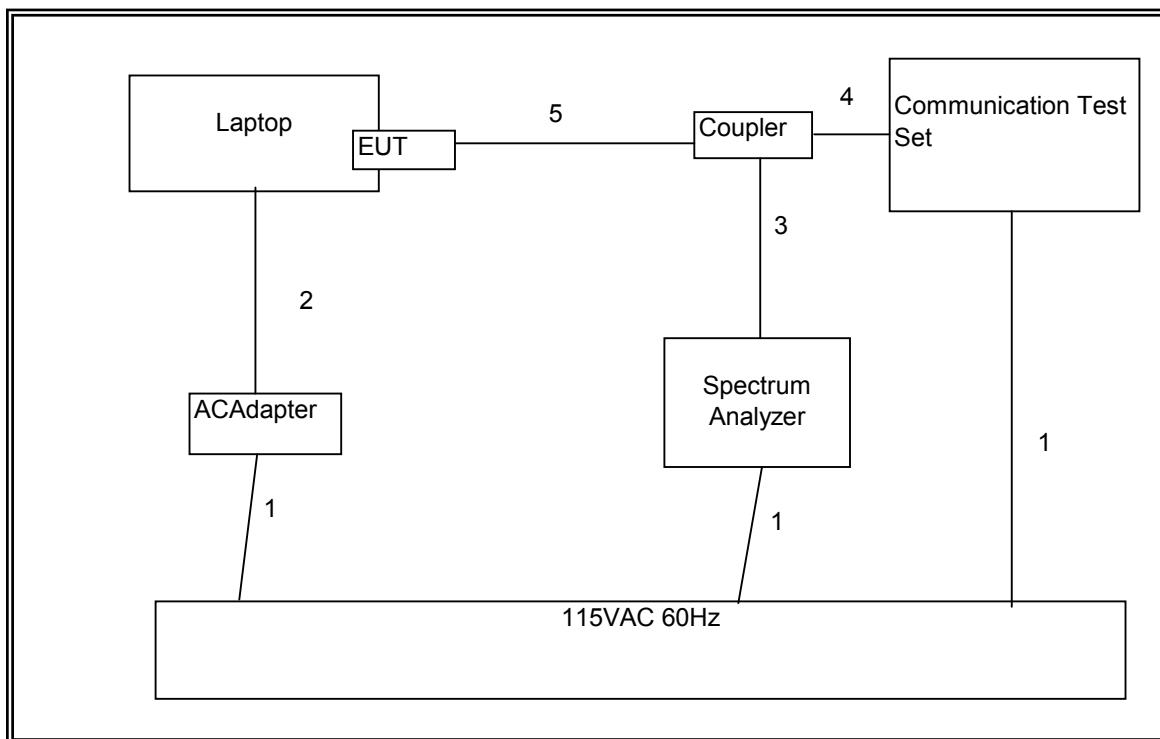
**SETUP DIAGRAM FOR RADIATED TESTS**
