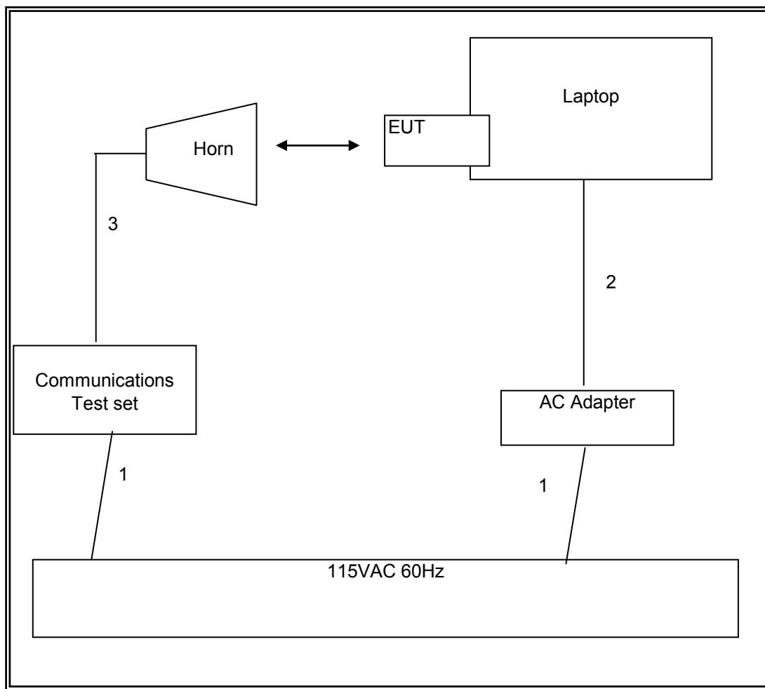
**SETUP DIAGRAM FOR RADIATED TESTS WITH EXTERNAL ANTENNA**
