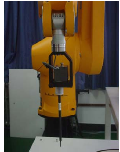
Picture3:EX3DV4 E-field probe
