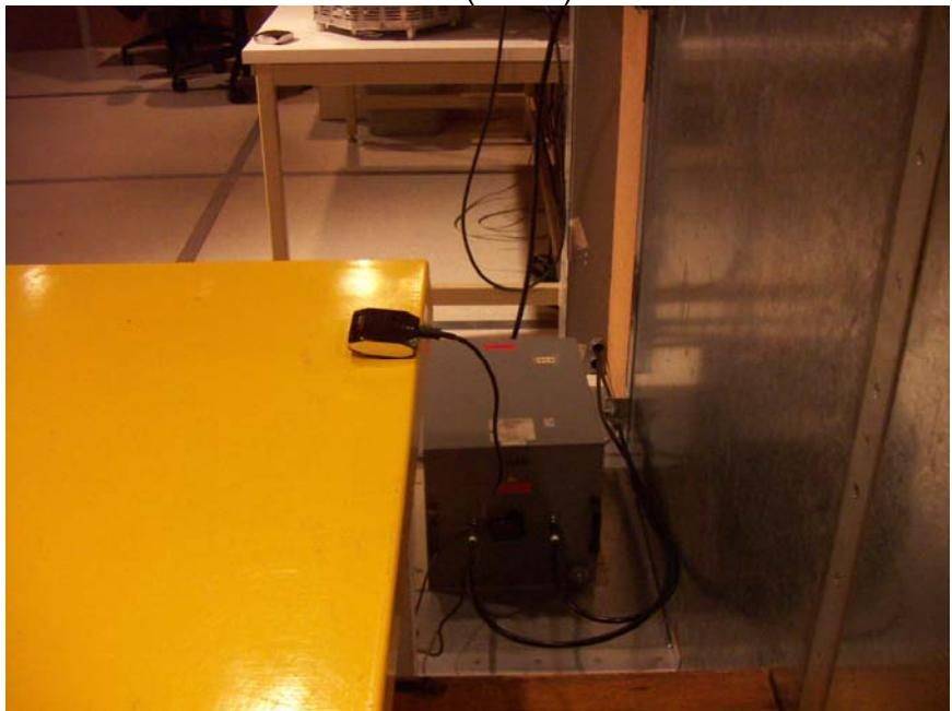
**AC MAINS LINE CONDUCTED EMISSION (EUT With Laptop Via USB Cable Link Mode)**
