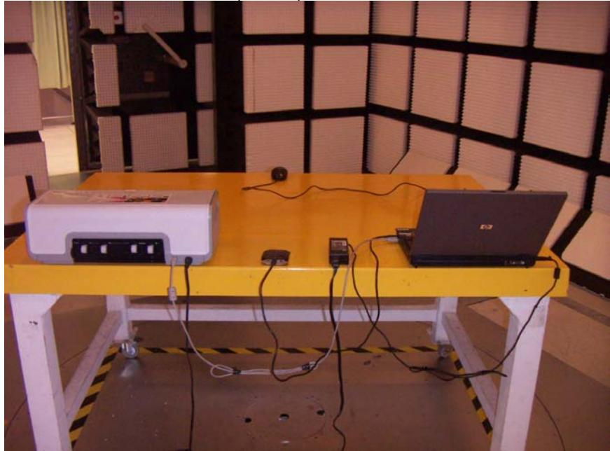
**AC MAINS LINE CONDUCTED EMISSION (EUT With AC Adapter Mode)**
