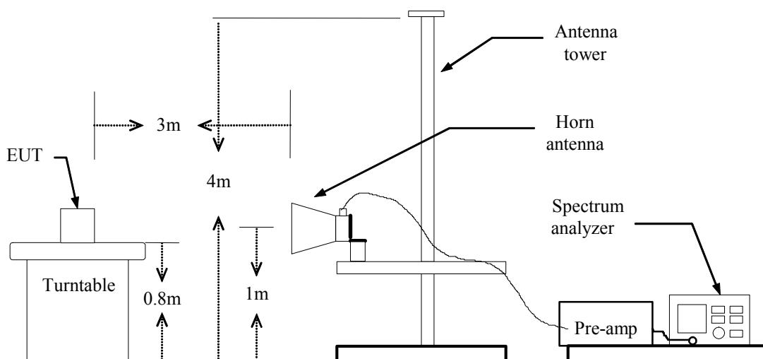
**For Substituted Method Test Set-UP**
