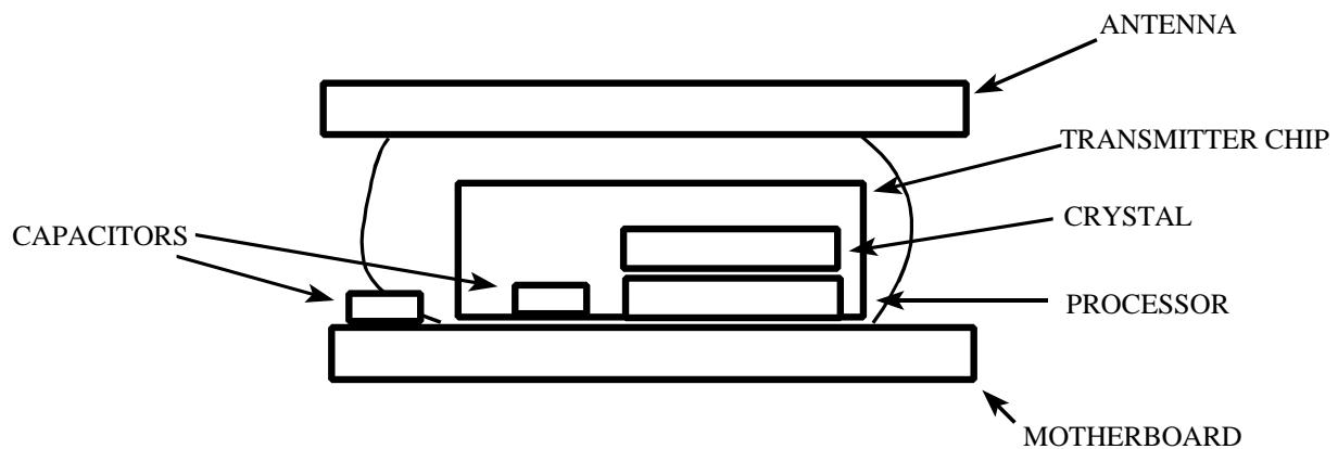
This diagram is included as part of the photograph submission for this application in order to clarify the assembly of this device. Due to the relatively small size of the product (less than 2 cm in diameter) clear photographs of this product are very difficult.
