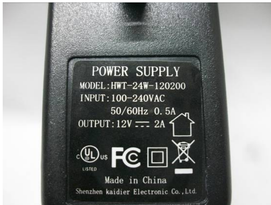
LABEL OF POWER SUPPLY-MODEL 1
