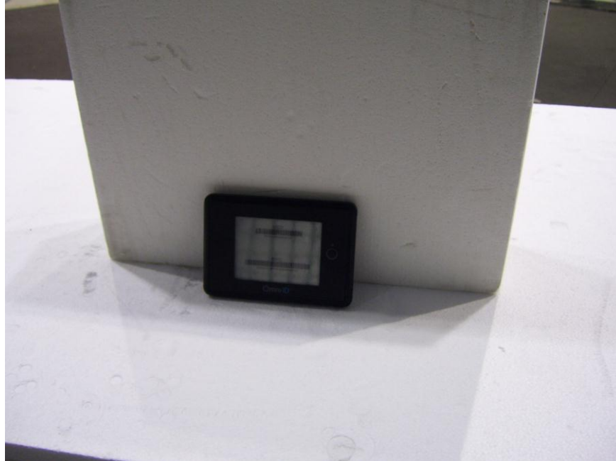
Figure 1: Radiated Emissions (worst case) all positions were tested for highest emissions
