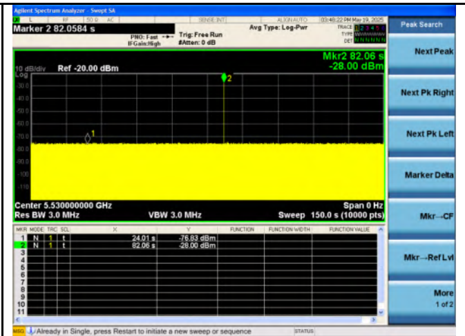
Radar at end of CAC - 5530MHz
