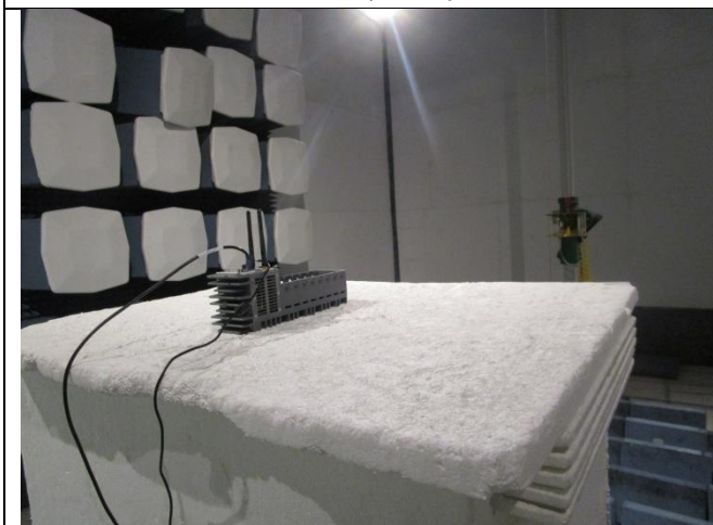
Radiated Emissions (>1GHz) – Front View
