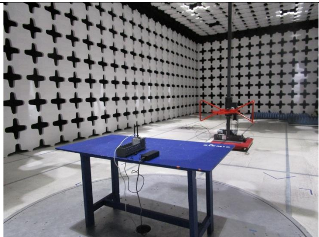
Radiated Emissions (<1GHz) – Rear View
