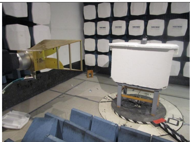
Radiated Emissions (>1GHz) – Rear View
