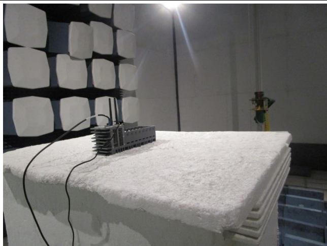
Radiated Emissions (>1GHz) – Front View
