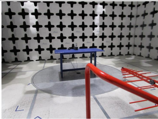
Radiated Emissions (<1GHz) – Front View
