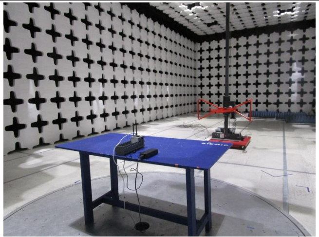
Radiated Emissions (<1GHz) – Rear View
