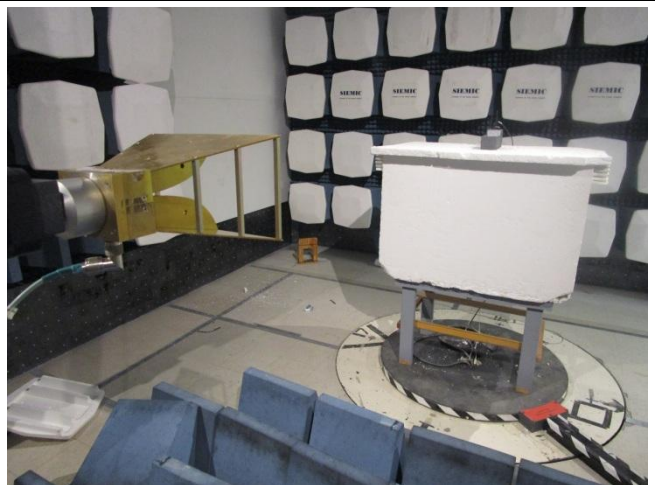
Radiated Emissions (>1GHz) – Rear View
