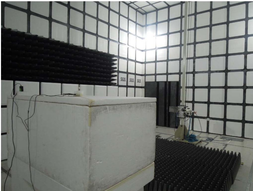
**Radiated Emission Set up Photos (Front View)**
