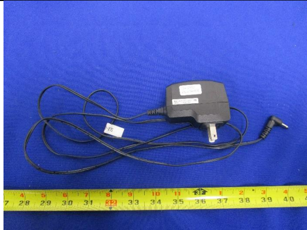
EUT Power Supply
