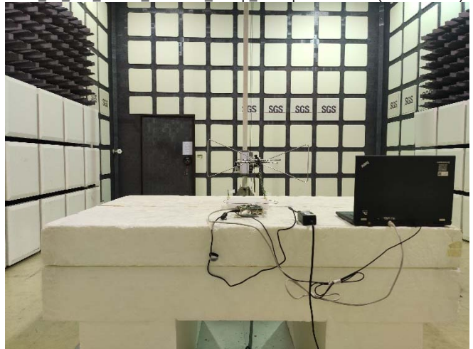
FCC_15_407_WLAN_Radiated_Setup_Monopole antenna (GW.05.0153)
