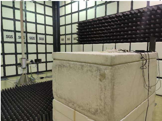
FCC_15_407_WLAN_Radiated_Setup_Monopole antenna (GW.05.0153)
