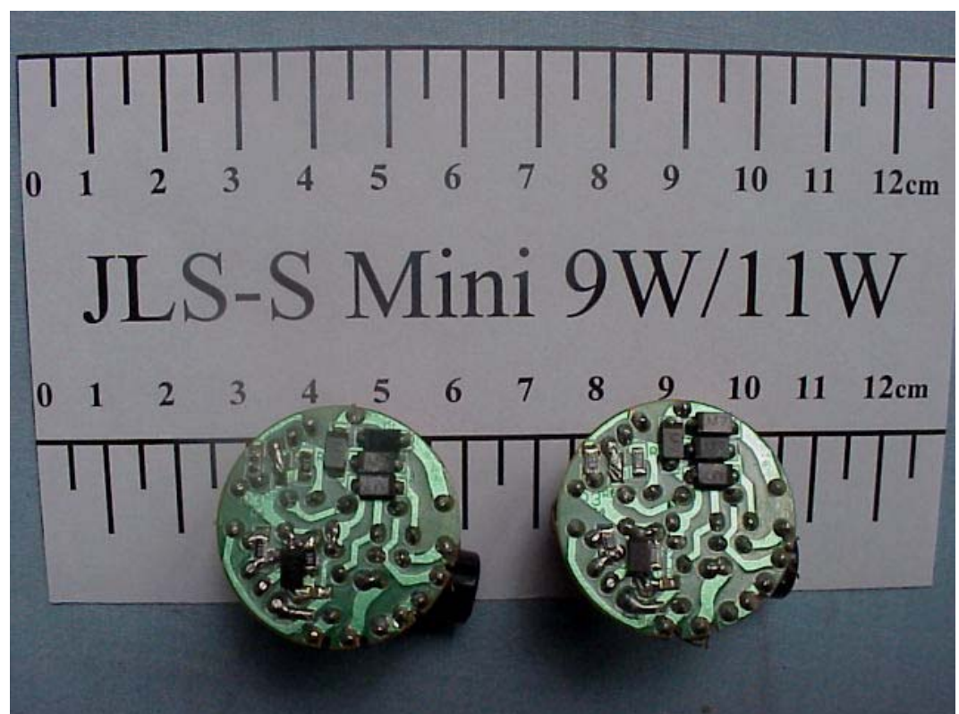
FIGURE 6 ENERGY SAVING LAMP (M/N: JLS-S Mini 9W/11W) MAIN BOARD (SOLDERED SIDE)
