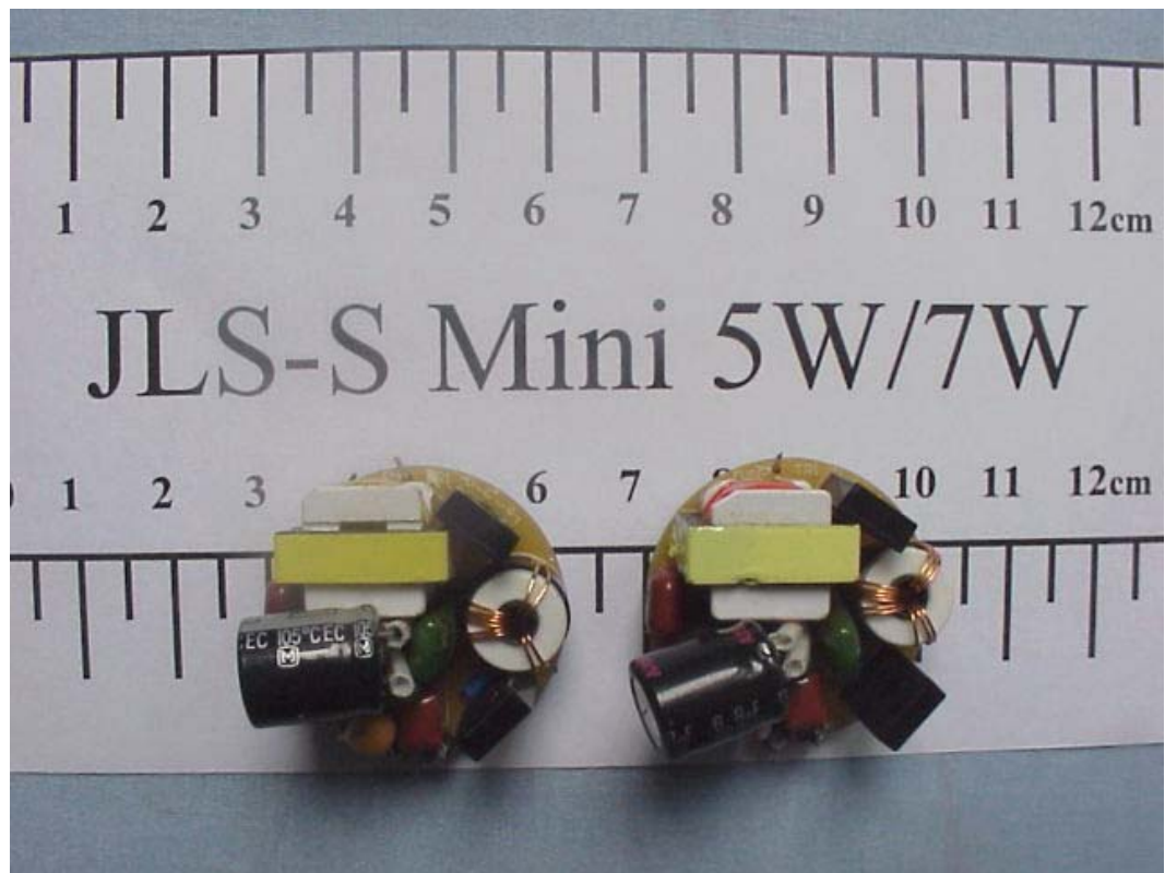
FIGURE 2 ENERGY SAVING LAMP (M/N: JLS-S Mini 5W/7W) MAIN BOARD (COMPONENT SIDE)
