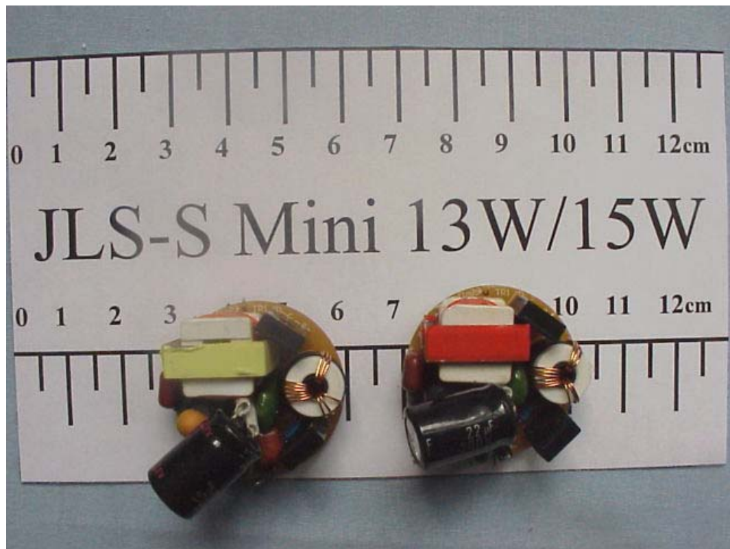
FIGURE 8 ENERGY SAVING LAMP (M/N: JLS-S Mini 13W/15W) MAIN BOARD (COMPONENT SIDE)
