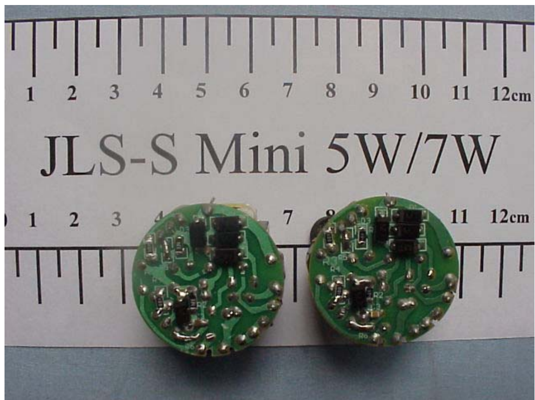
FIGURE 3 ENERGY SAVING LAMP (M/N: JLS-S Mini 5W/7W) MAIN BOARD (SOLDERED SIDE)
