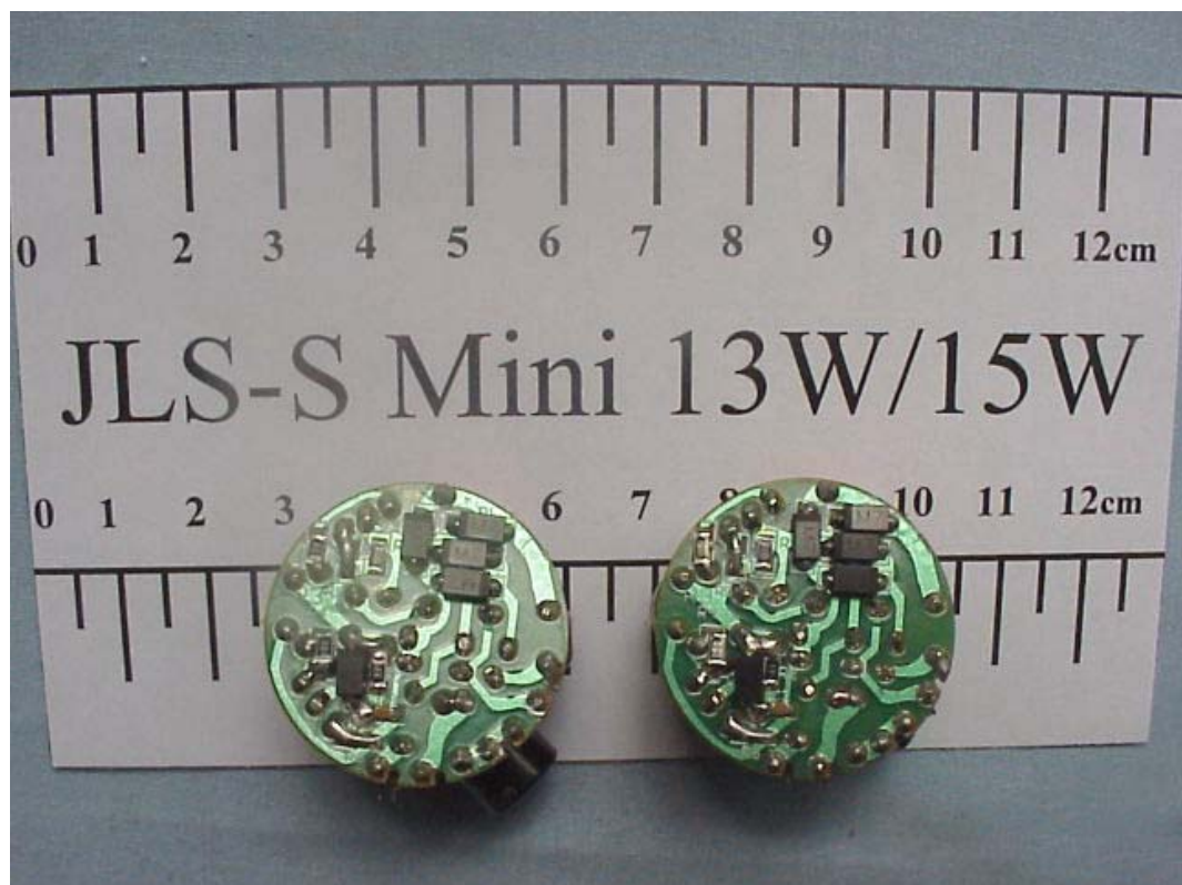
FIGURE 9 ENERGY SAVING LAMP (M/N: JLS-S Mini 13W/15W) MAIN BOARD (SOLDERED SIDE)
