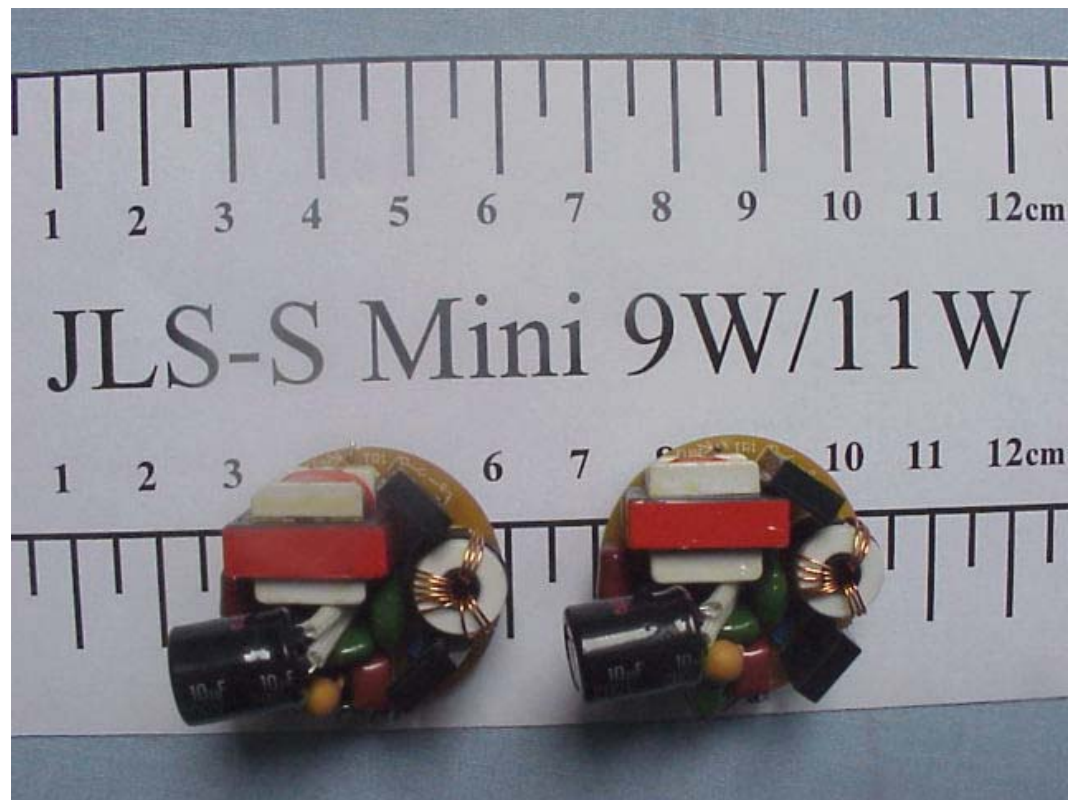
FIGURE 5 ENERGY SAVING LAMP (M/N: JLS-S Mini 9W/11W) MAIN BOARD (COMPONENT SIDE)
