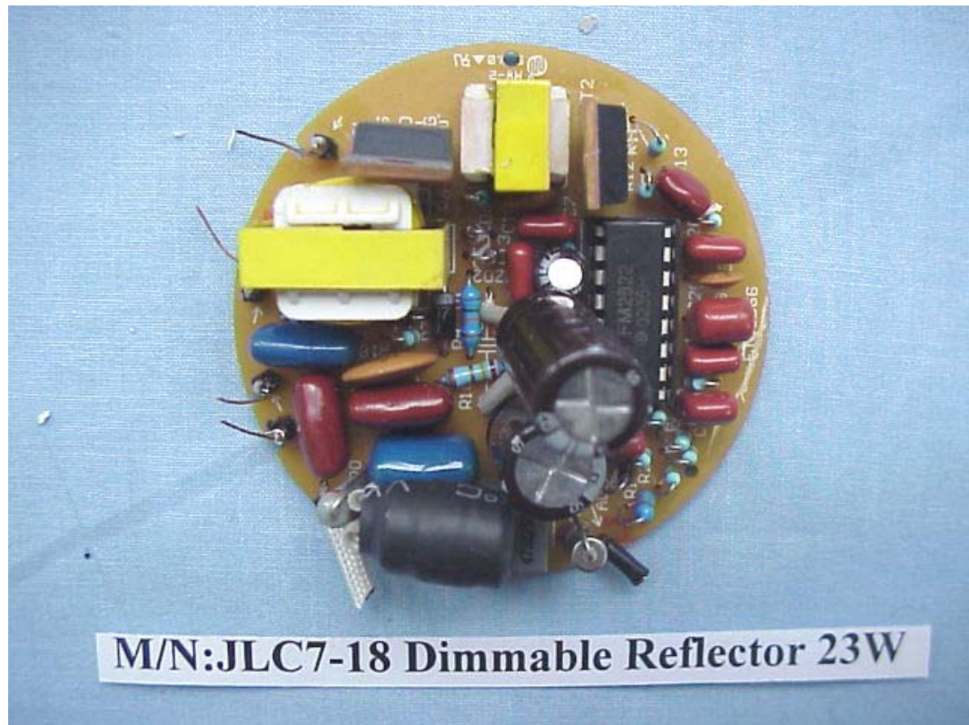
FIGURE 11 ENERGY SAVING LAMP (M/N: JLC7-18 DIMMABLE REFLECTOR 23W) MAIN BOARD (COMPONENT SIDE)
