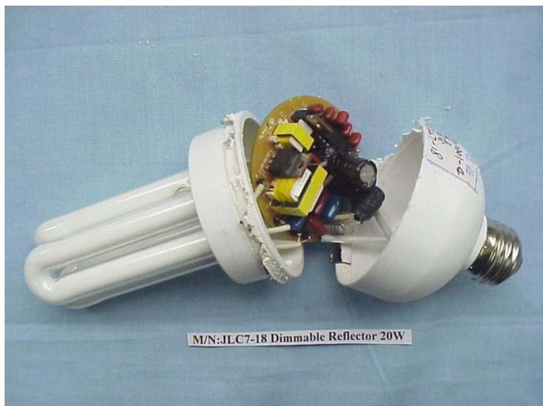
FIGURE 6 ENERGY SAVING LAMP (M/N: JLC7-18 DIMMABLE REFLECTOR 20W) COVER REMOVED 2
