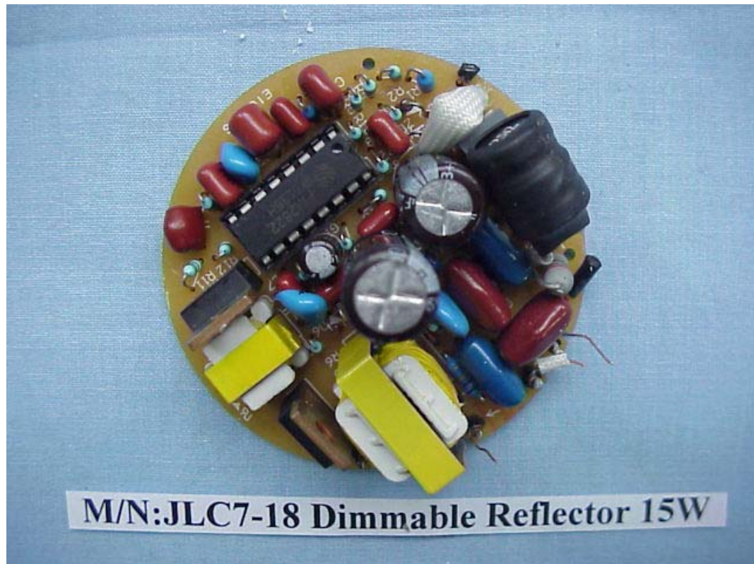
FIGURE 3 ENERGY SAVING LAMP (M/N: JLC7-18 DIMMABLE REFLECTOR 15W) MAIN BOARD (COMPONENT SIDE)
