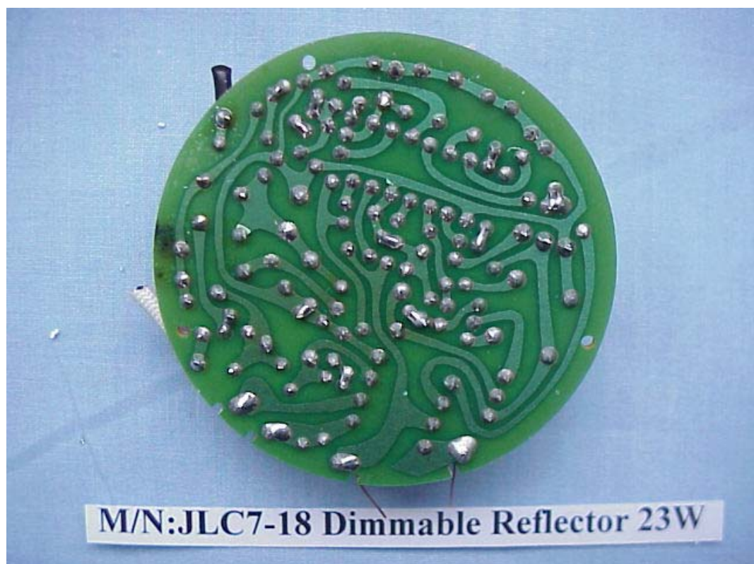
FIGURE 12 ENERGY SAVING LAMP (M/N: JLC7-18 DIMMABLE REFLECTOR 23W) MAIN BOARD (SOLDERED SIDE)
