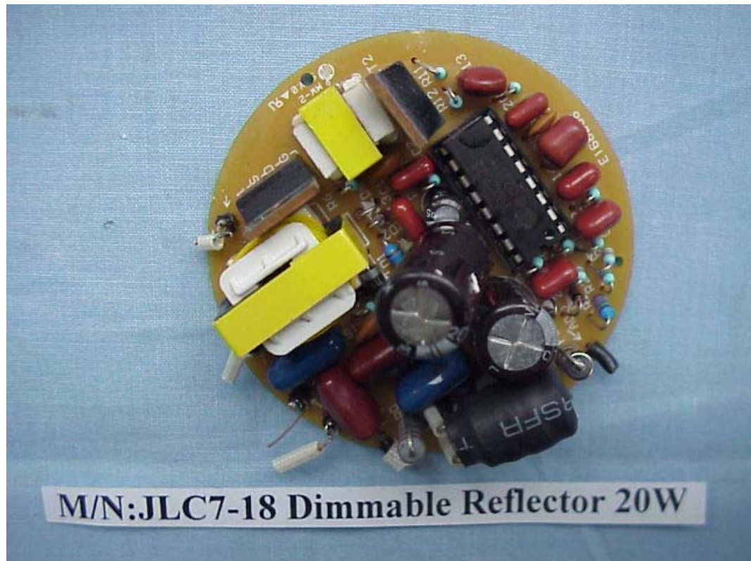
FIGURE 7 ENERGY SAVING LAMP (M/N: JLC7-18 DIMMABLE REFLECTOR 20W) MAIN BOARD (COMPONENT SIDE)
