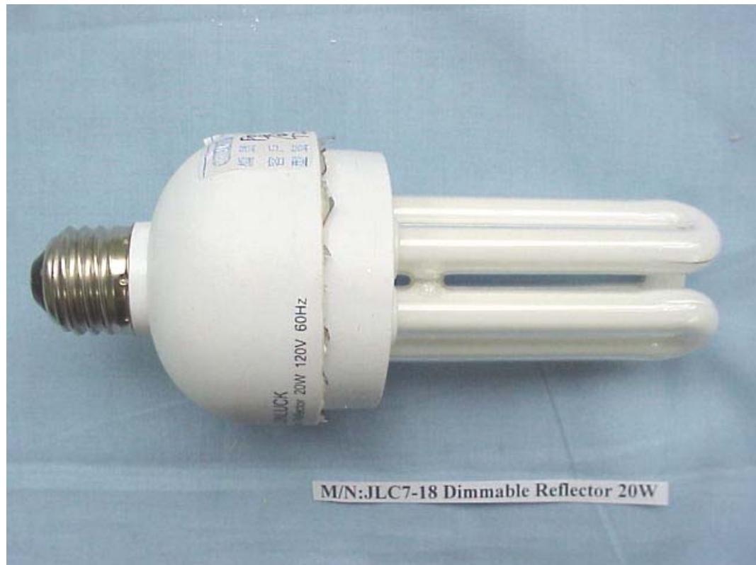
FIGURE 5 ENERGY SAVING LAMP (M/N: JLC7-18 DIMMABLE REFLECTOR 20W) COVER REMOVED 1
