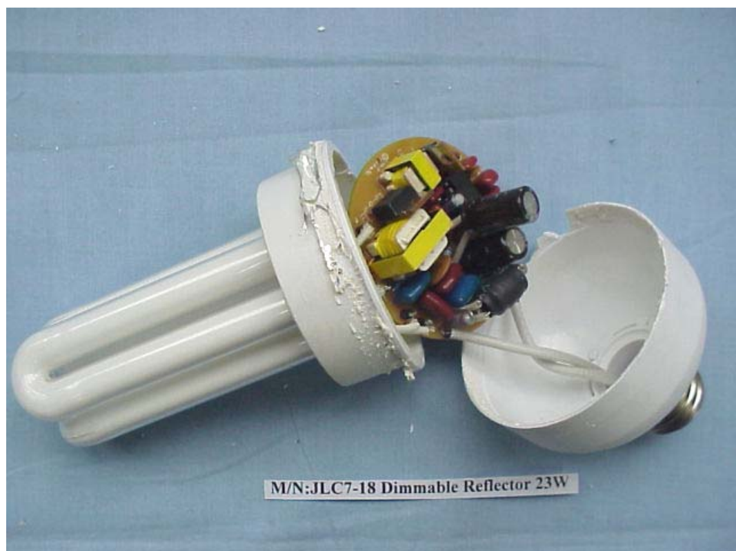
FIGURE 10 ENERGY SAVING LAMP (M/N: JLC7-18 DIMMABLE REFLECTOR 23W) COVER REMOVED 2
