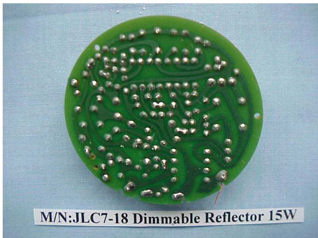
FIGURE 4 ENERGY SAVING LAMP (M/N: JLC7-18 DIMMABLE REFLECTOR 15W) MAIN BOARD (SOLDERED SIDE)
