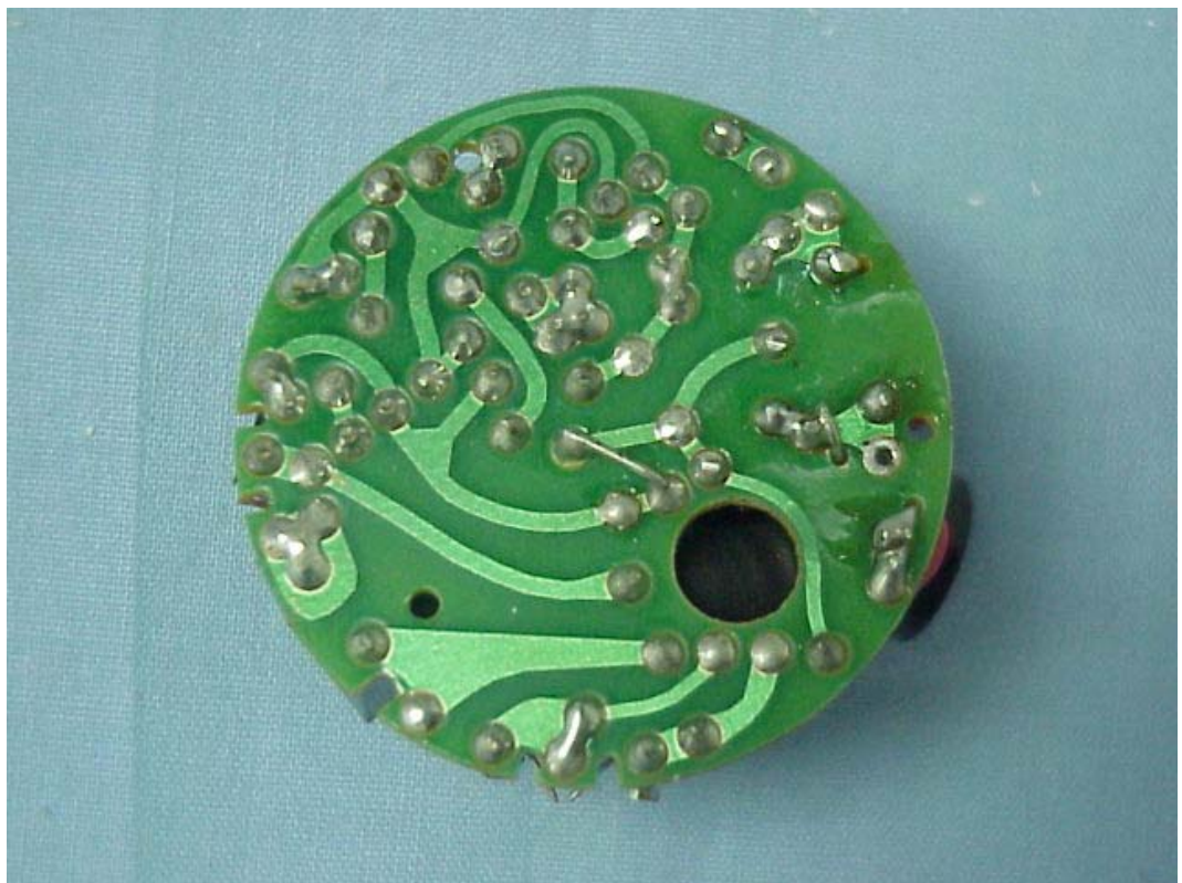
FIGURE 6 ELECTRONIC ENERGY SAVING LAMP (M/N: JLC7-18 GLOBE 9W) MAIN BOARD (SOLDERED SIDE)
