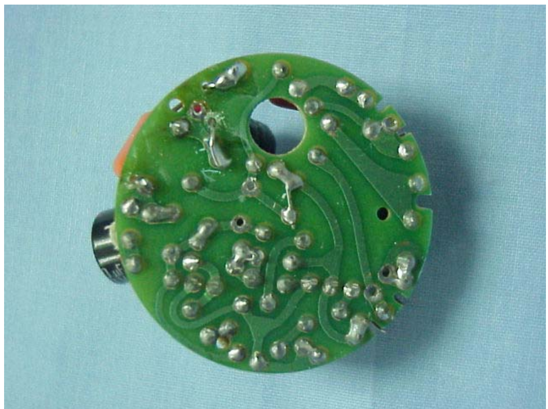
FIGURE 3 ELECTRONIC ENERGY SAVING LAMP (M/N: JLC7-18 A-TYPE 9W) MAIN BOARD (SOLDERED SIDE)
