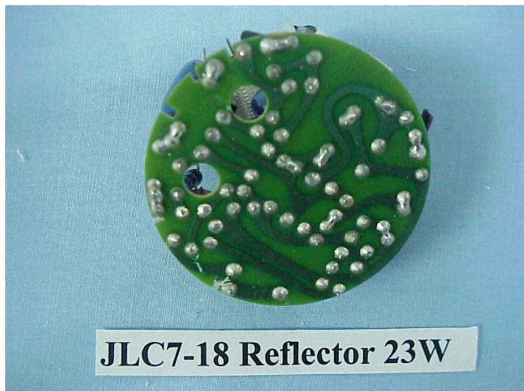
FIGURE 3 ELECTRONICS ENERGY SAVING LAMP (M/N: JLC7-18 REFLECTOR 23W) MAIN BOARD (SOLDERED SIDE)
