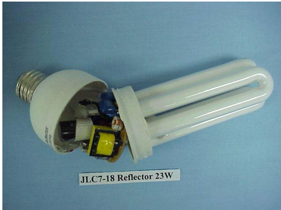
FIGURE 1 ELECTRONICS ENERGY SAVING LAMP (M/N: JLC7-18 REFLECTOR 23W) COVER REMOVED
