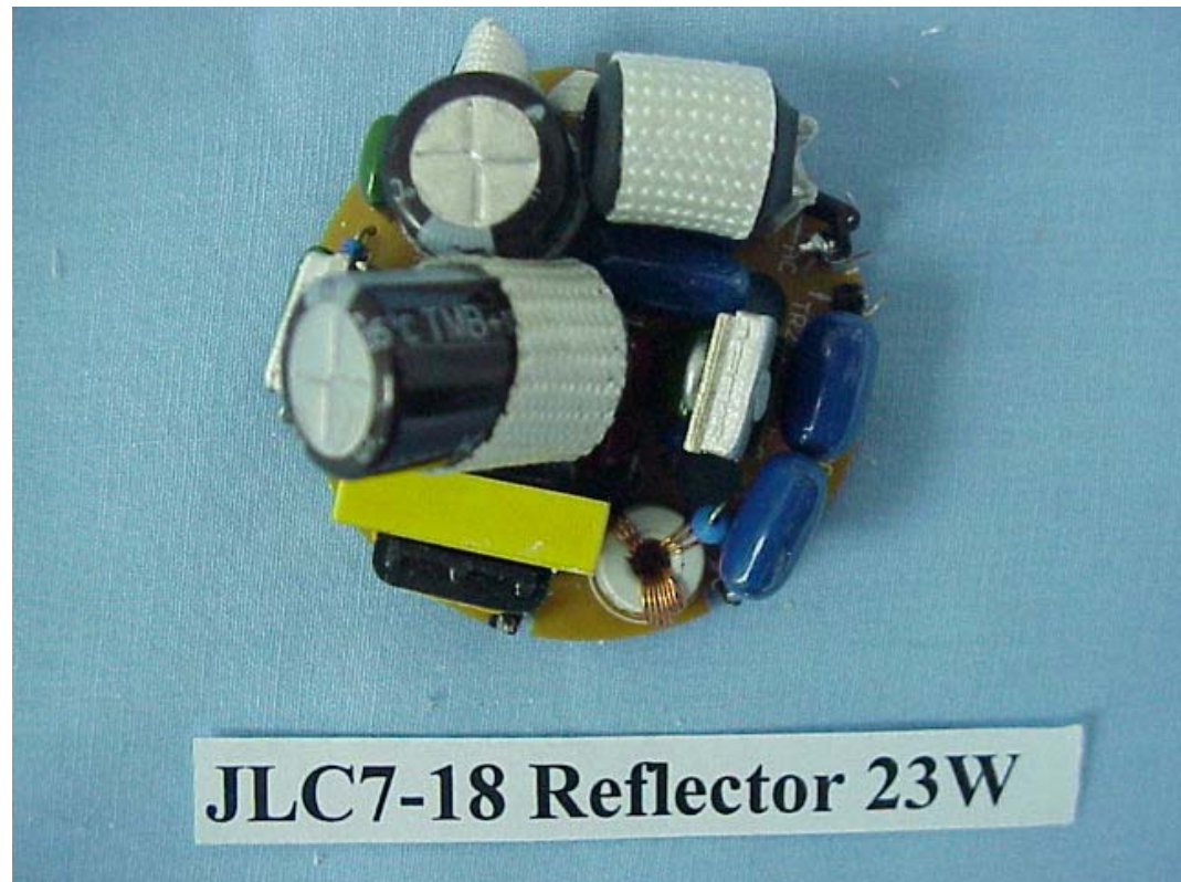
FIGURE 2 ELECTRONICS ENERGY SAVING LAMP (M/N: JLC7-18 REFLECTOR 23W) MAIN BOARD (COMPONENT SIDE)
