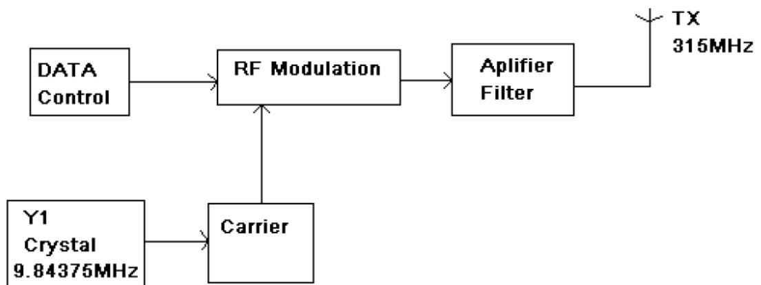
TX module receives the data from the MCU, then modulate the data to carry frequency 315MHZ, and at last emit the carrier signal from the antenna.
