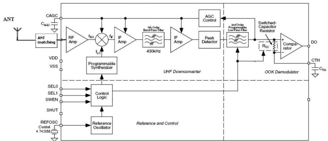
It is consisted with four sections: Ant matching net working, UHF downconverter, Resference and control, and OOK demodulator. Also shown in the figure are two capacitors (CTH, CAGC) and one timing component, usually a crystal. With the exception of a supply decoupling capacitor, and antenna impedance matching network, these are the only external components needed to assemble a complete UHF receiver.
