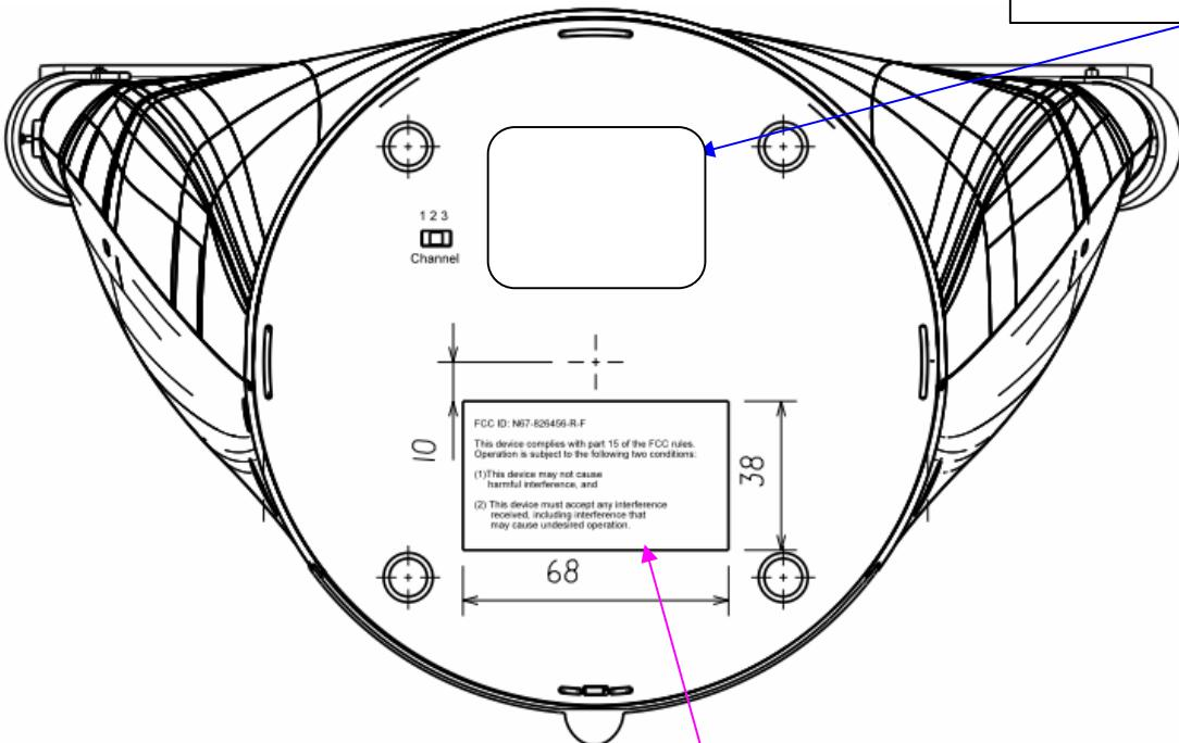
**FCC Information is set here which was made by an insert part on the mould.**
