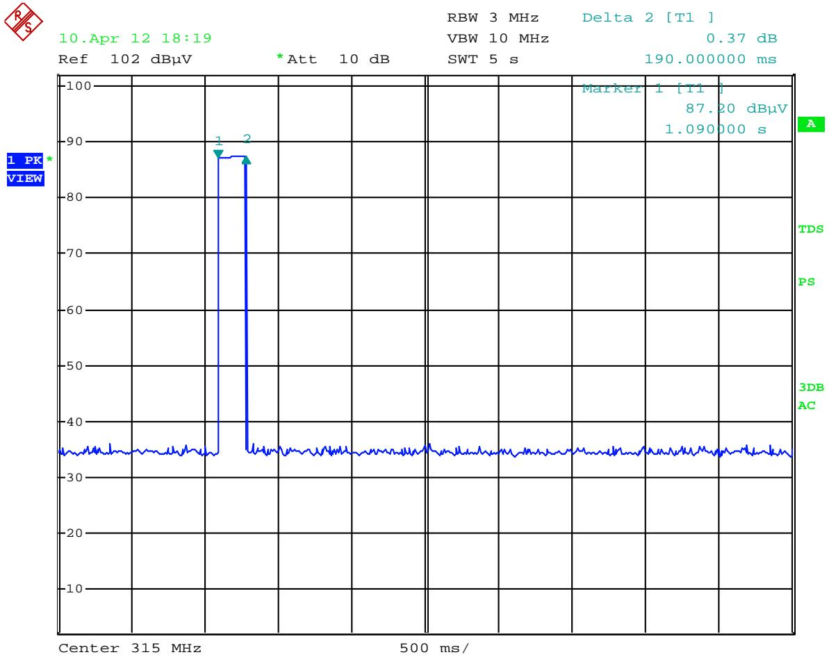
The controller is a manually operated transmitter, it employs a switch that will automatically deactivate the transmitter within not more than 5 seconds of being released.
