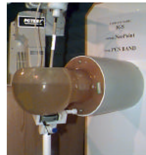
Figure 1. SAR Test Set-up
