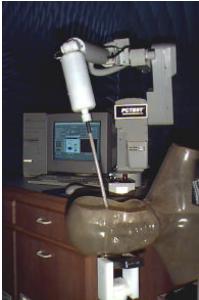
Figure 5. Photograph of the Probe and the Phantom
