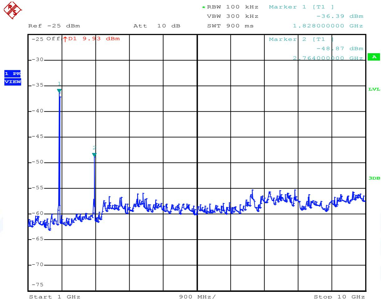
Note: Signal level no. 2 is located in restricted band (2690 – 2900 MHz).
