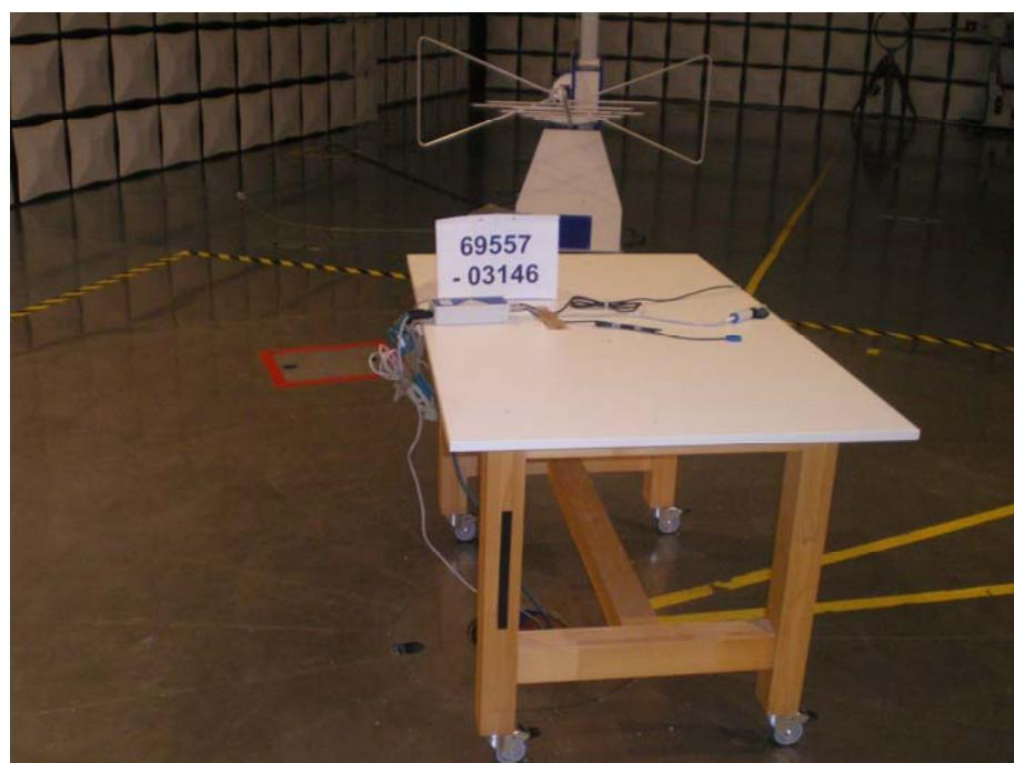
**Test setup for radiated emission measurement
