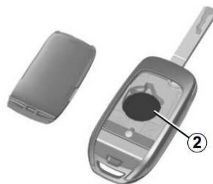
**Note:** It is not advisable to touch the electronic circuit in the key cover when replacing the battery.
