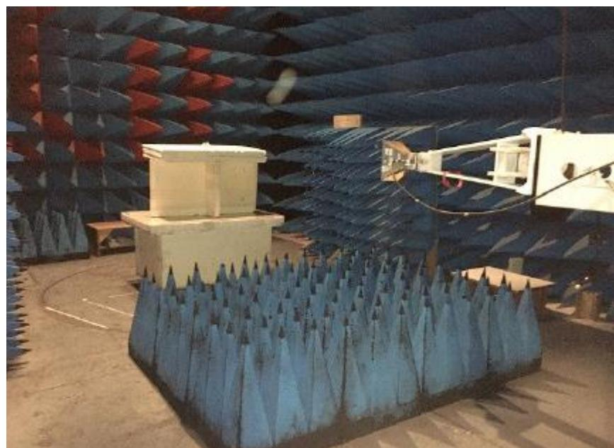
**Radiated emissions measurements setup**
