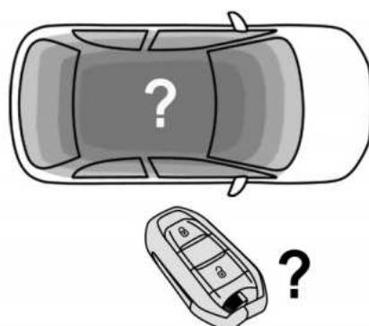
When the electronic key is not detected or is no longer in the detection zone, a message appears on the remote device when closing a door or when requesting engine switch-off.
