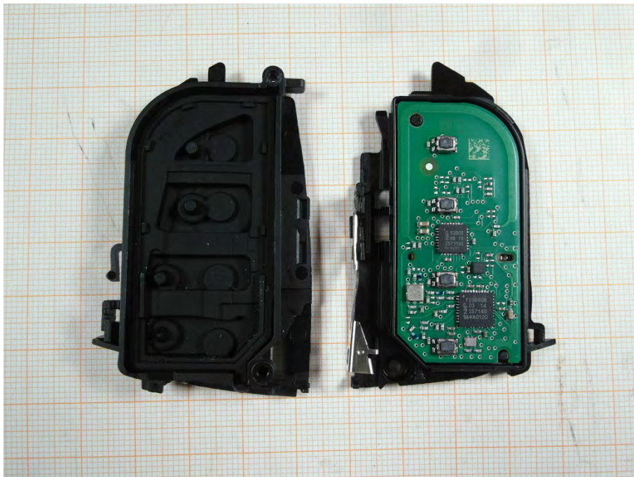
Photo 10: internal PCB, EN and FCC/IC version, chrome variant
