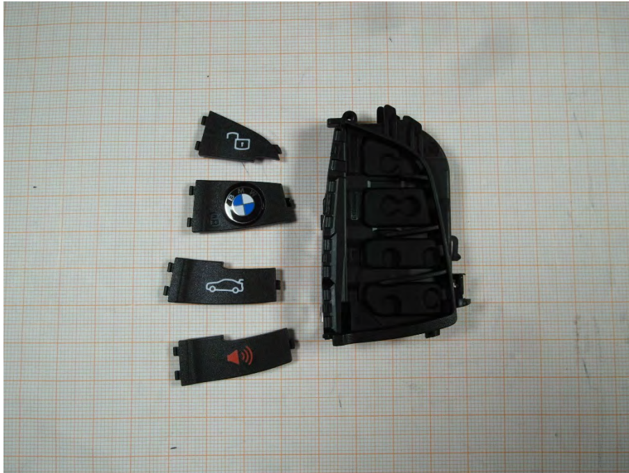
Photo 24: buttons removed, FCC/IC version
