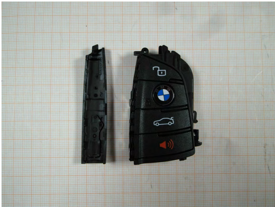
Photo 23: button holder removed, FCC/IC version
