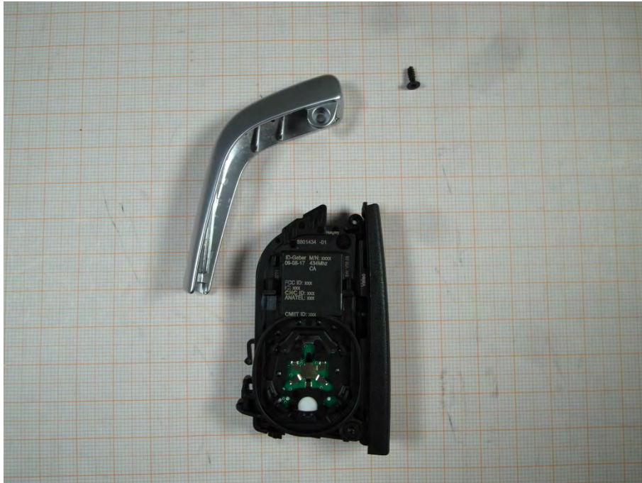
Photo 18: screws released, metal peace removed
