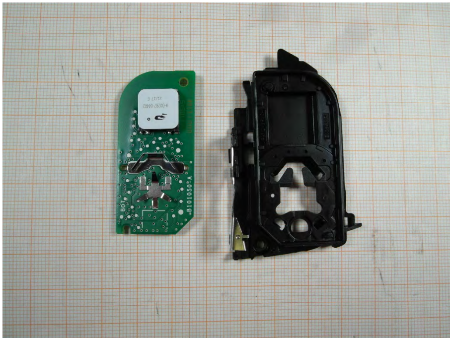
Photo 12: internal PCB, EN and FCC/IC version, chrome variant
