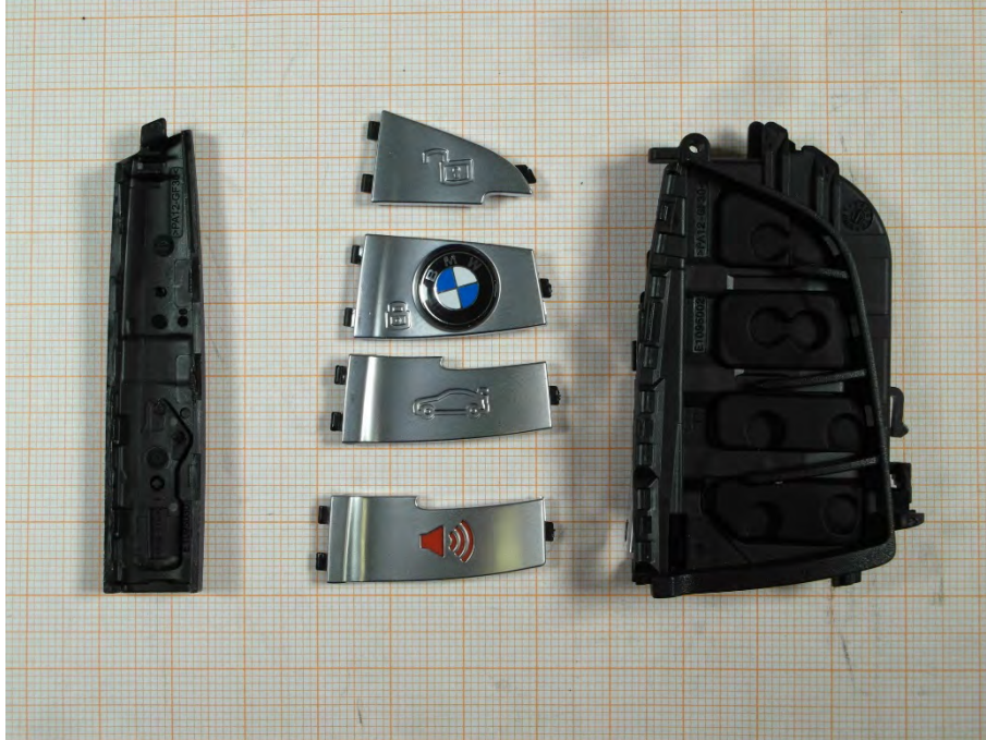
Photo 9: buttons removed, FCC/IC version
