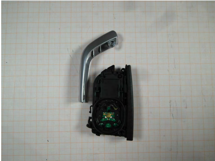
Photo 22: metal peace removed, FCC/IC version
