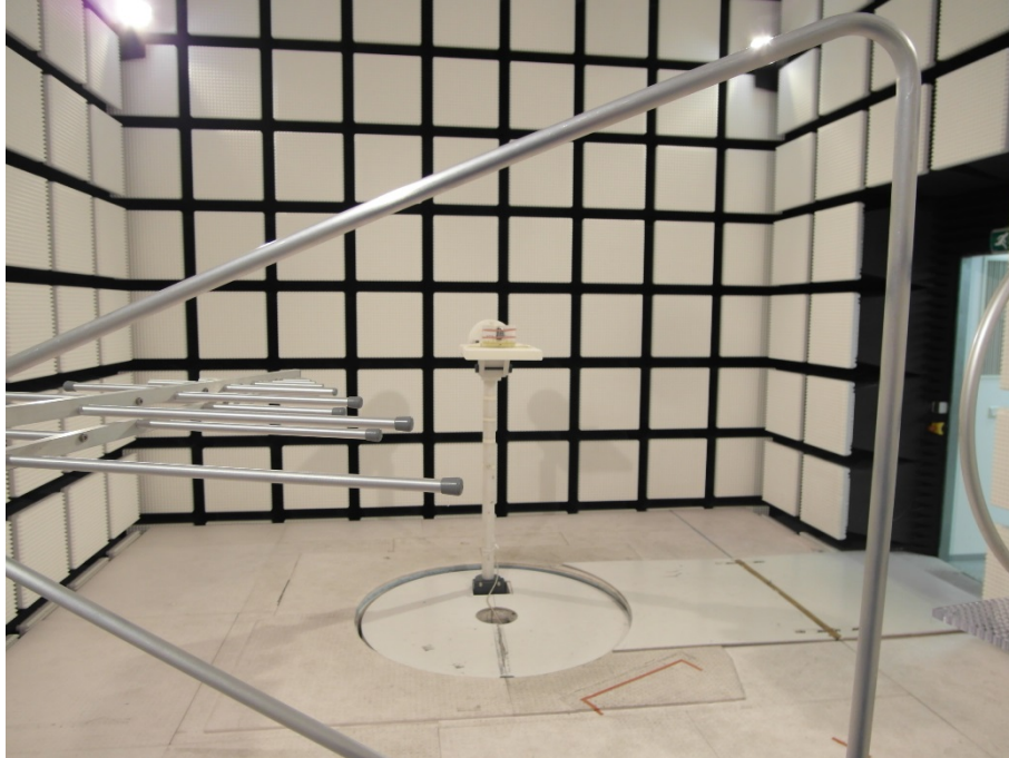
Photo 5: chrome variant 3m fully anechoic chamber
