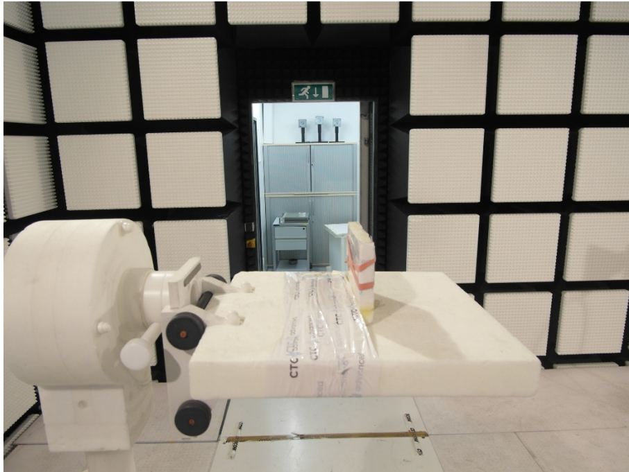
Photo 15: black variant 3m fully anechoic chamber
