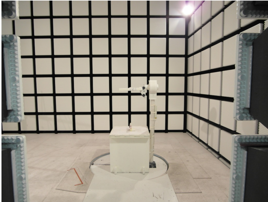
Photo 7: chrome variant 3m magnetic measurements
